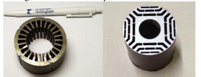
Fig. 18. Stator and rotor laminations [96].
