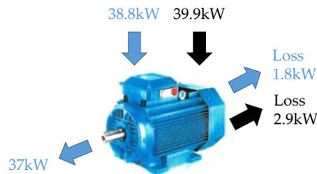
Fig. 21. Losses and motor efficiency of the ABB's 37kW SCIM and the equivalent SynRM at rated conditions. (SynRM highlighted with blue, SCIM highlighted with black).
