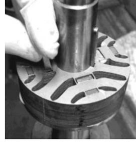
Fig. 13. PM insertion. SynRM to PMaSynRM [91].
