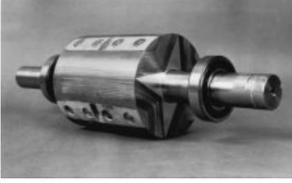
Fig. 10. Assembled ALA rotor topology. [73]
