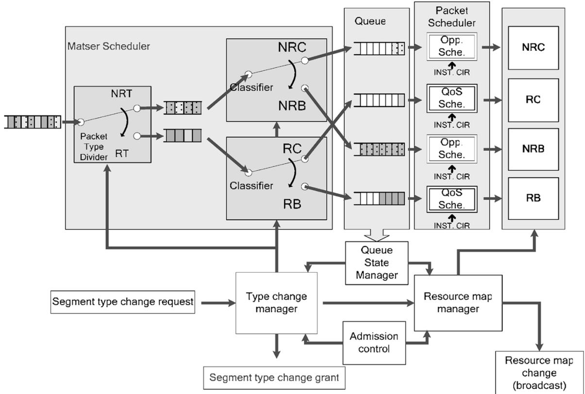
Fig. 8. Segment allocation in the designed DiffSeg system.
