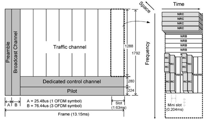
Fig. 4. Frame structure of the designed DiffSeg system.
