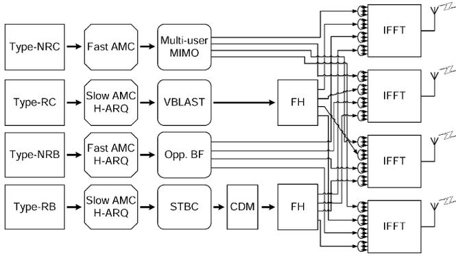
Fig. 5. Basic structure of the designed DiffSeg transmitter.
