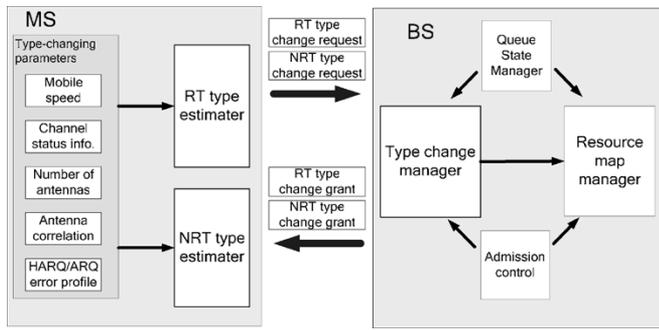
Fig. 6. Mobile-assisted classification of the segment type.
