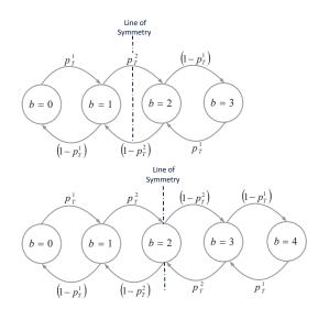
Fig. 6. Finite state diagrams for battery-conditioned energy management policies with battery capacities K = 3 and K = 4. Symmetric and complementary transition probabilities are illustrated for the computation of the minimum information leakage rate in case of an equiprobable input load, i.e.,  $p_x = 0.5$ .
