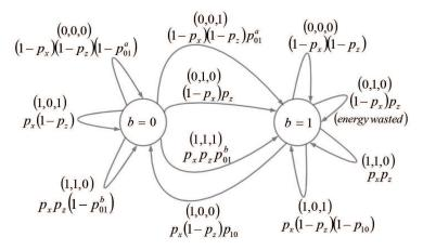
Fig. 2. Finite state diagram for the battery conditioned energy management policy with s = 2 states. Each triplet in the figure corresponds to the (x, z, y) values for the corresponding transition. Transition probabilities are also included in the figure.
