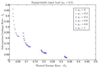
Fig. 5. The Pareto optimal  $(I_p, E_w)$  pairs for  $p_x = 0.5$  and for different  $p_z$  values. Optimal pairs for different  $p_z$  values are illustrated with different markers.
