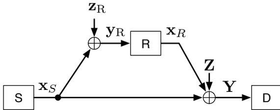
Fig. 2. Half-Duplex Binary Input Gaussian Relay Channel
