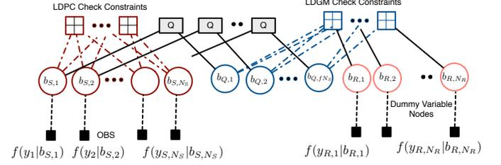
Fig. 6. Simplified factor graph with one-bit scalar quantizer and DBLAST.
