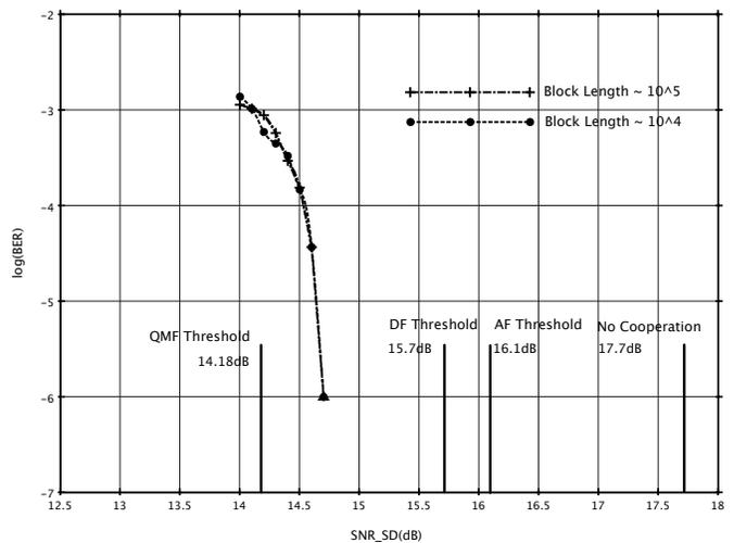
(b) BER simulation for  $\mathbf{b}_R$  using design rate of 5.4bits/sec/Hz with 64QAM.
