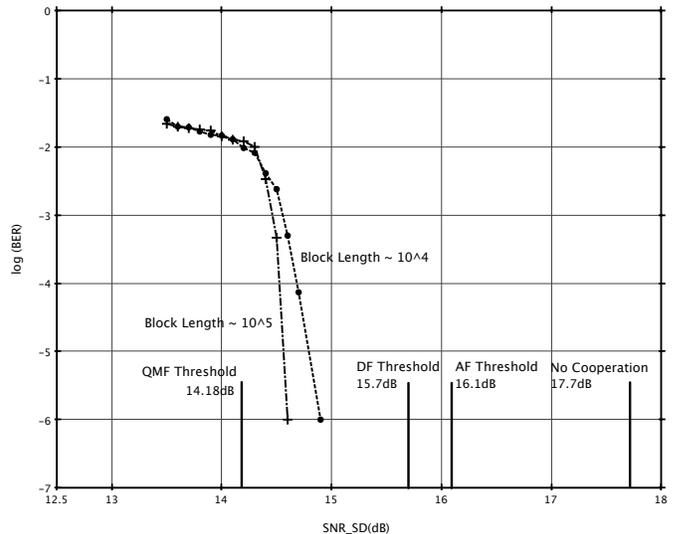
(a) BER for  $\mathbf{b}_S$  using design rate of 5.4bits/sec/Hz with 64QAM.
