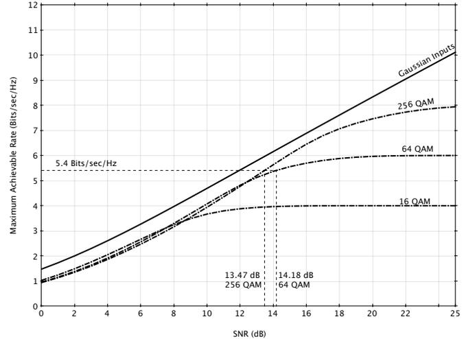
Fig. 11. Maximum achievable rate for QMF relaying with modulation constraints on channel inputs plotted vs  $\text{SNR}_{SD}$  for SNR relationships in Eq. (4)
