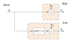
Fig. 3. Gaussian erasure wiretap channel: in the asymptotic case, the erasures/overflows at Eve's A/D due to the rapid power modulation at the transmitter can be modeled by an erasure channel.
