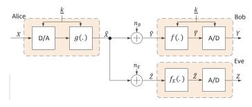
Fig. 1. The message X is observed at Bob and Eve through the transmitter, the AWGN channels with different noise variances, and their respective receivers with (possibly nonlinear) functions g(.), f(.), and  $f_E(.)$ . The sequence  $\underline{k}$  is a cryptographic key shared by Alice and Bob, which is assumed to be obtained by Eve immediately *after* she has recorded Z.
