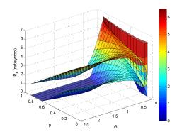
Fig. 7. Achievable secrecy rate vs. the probability p and the gain at Eve's receiver, G for the case of noiseless channels. The ratio between the two power levels at the transmitter is  $r = 10^3$  (i.e. 30 dB) and the average transmitting power is P = 1. In the upper curve, both Bob and Eve have the same 10-bit A/D's. In the lower curve, Bob uses a 10-bit A/D while Eve uses a 14-bit A/D (Eve's A/D is 24 dB better than Bob's A/D) and a maxi-min rate of  $R_s = 1.2478$  is achieved (for p = 0.4).
