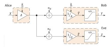
Fig. 2. Alice and Bob share a cryptographic key that determines the value of A at each time instance. Eve puts a (possibly variable) gain before her A/D to decrease the A/D erasures and/or overflows and hence increase the information leakage.
