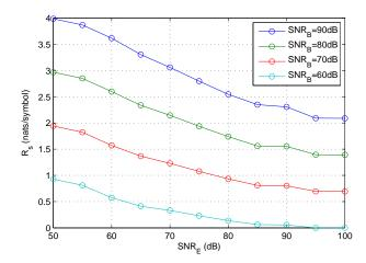
Fig. 9. Achievable secrecy rates for various values of the SNR at Bob's receiver when the SNR at Eve's receiver changes from 50 dB to 100 dB. The settings are  $r = 10^3$ , P = 1, and Bob and Eve are applying 10-bit A/D's. When the SNR of the channel between Alice and Eve is significantly better than the SNR of the channel between Alice and Bob, reasonable secrecy rates are still achievable.
