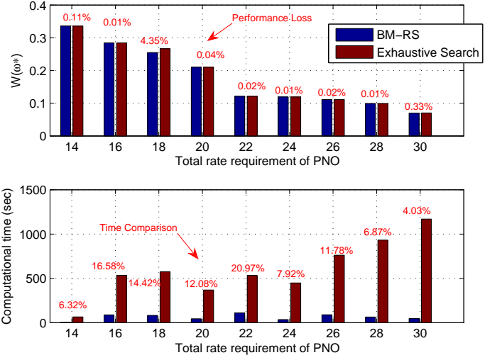
Fig. 11: Performance of Algorithm (BM-RS) under different R_0^{\text{req}} . Top plot: Value of W(w^*) ; Bottom plot: Computational time.
