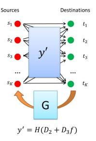
Fig. 5. Phase 3: Now each source has two sets of signals x and f, and sources can send out a linear combination of x and f to destinations via the forward channel. Destinations get  $y' = H(D_2x + D_3f) + \text{noise}$ .
