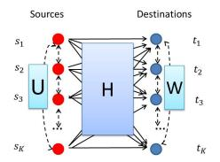
Fig. 2. System Model For In-Band Interaction:  $s_1, s_2, \ldots, s_K$  are sources and  $t_1, t_2, \ldots, t_K$  are destinations. *H* is the forward channel matrix from sources to destinations, *U* is the channel matrix among sources, and *W* is the channel matrix among destinations.
