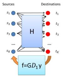
Fig. 4. Phase 2: After receiving signals from sources in phase1, all destinations scale y and send back to sources using the feedback channel. Sources get  $f = GD_1y +$ noise.
