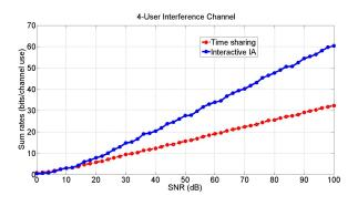
Fig. 7. Numeric Finite SNR Performance Simulations for 4-User Interference Channel with Out-of-Band Reverse (Feedback) Channel.
