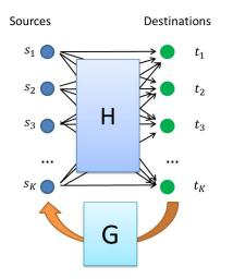
Fig. 1. System Model For Out-of-Band Interaction:  $s_1, s_2, \ldots, s_K$  are sources and  $t_1, t_2, \ldots, t_K$  are destinations. *H* is the forward channel matrix from sources to destinations, and *G* is the feedback channel matrix from destinations to sources.
