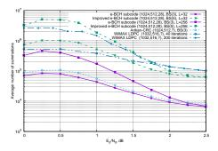
Figure 8: Decoding complexity for polar subcodes with Arikan kernel
