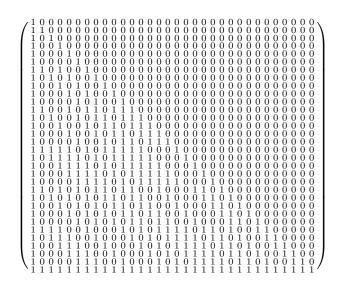
Figure 6: Extended BCH kernel  $F_{32}$
