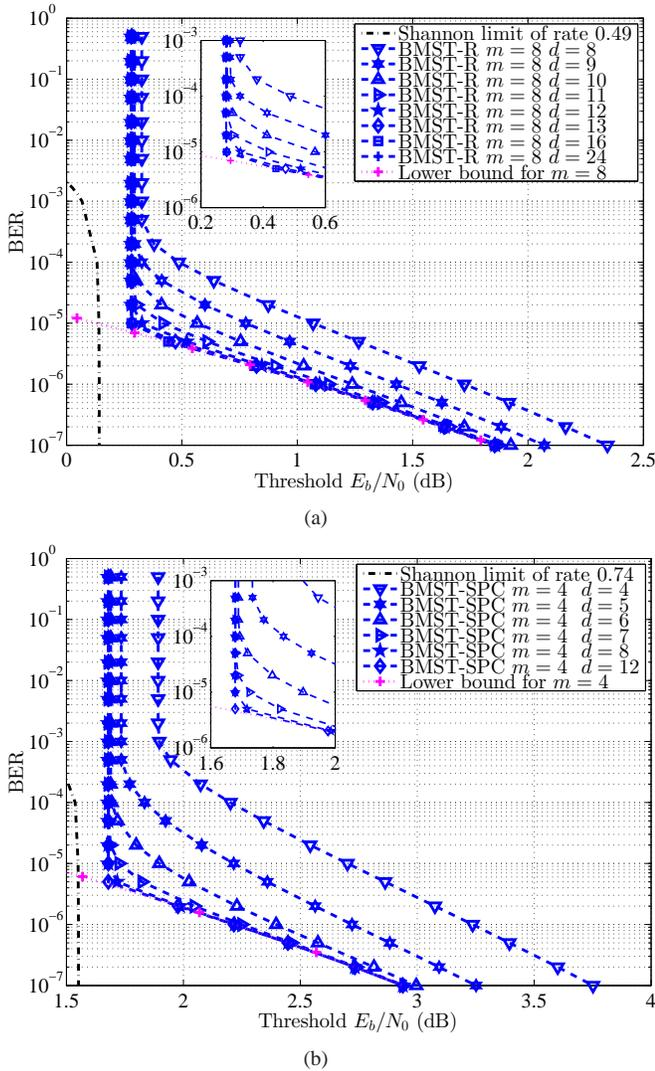
Fig. 5. Window decoding thresholds in terms of  $E_b/N_0$  (dB) with different target BERs and different decoding delays for (a) a rate  $R_{\text{BMST}} = 0.49$  BMST-R [2, 1] code ensemble with  $m = 8$  and  $L = 392$ , and (b) a rate  $R_{\text{BMST}} = 0.74$  BMST-SPC [4, 3] code ensemble with  $m = 4$  and  $L = 296$ .
