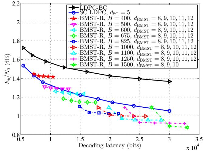
Fig. 12. Required  $E_b/N_0$  to achieve a BER of  $10^{-5}$  for (3,6)-regular LDPC-BCs, (3,6)-regular SC-LDPC codes, and BMST-R [2,1] codes as a function of decoding latency.
