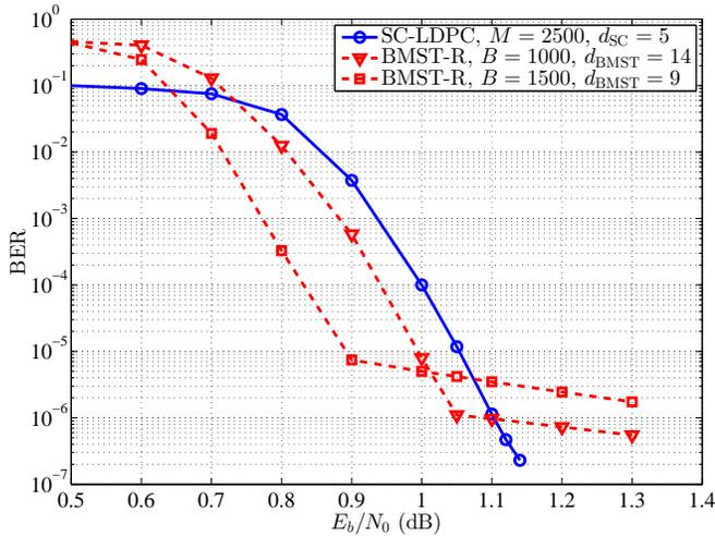
Fig. 11. Simulated decoding performance of BMST-R [2,1] codes with encoding memory  $m = 8$  compared to (3,6)-regular SC-LDPC code with coupling width  $m = 1$ . The values of  $B$  and  $d_{\text{BMST}}$  for the BMST-R codes are chosen in such a way that the decoding latencies of all the codes are the same.
