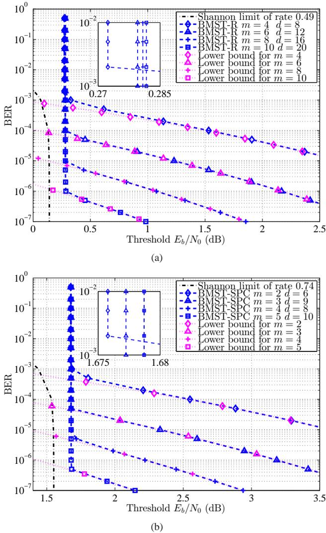
Fig. 9. Window decoding thresholds in terms of  $(E_b/N_0)^*$  (dB) with different target BERs for two BMST code ensemble families with different encoding memories  $m$ . (a) BMST-R [2, 1] code ensemble and (b) BMST-SPC [4, 3] code ensemble.
