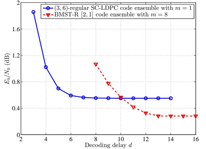
Fig. 6. Window decoding thresholds for a (3, 6)-regular SC-LDPC code ensemble with  $m = 1$  and a BMST-R [2, 1] code ensemble with  $m = 8$  as a function of decoding delay  $d$ . The preselected target BER is  $10^{-5}$ . The component submatrices for the SC-LDPC code ensemble are  $\mathbf{B}_0 = [2 \ 1]$  and  $\mathbf{B}_1 = [1 \ 2]$ .
