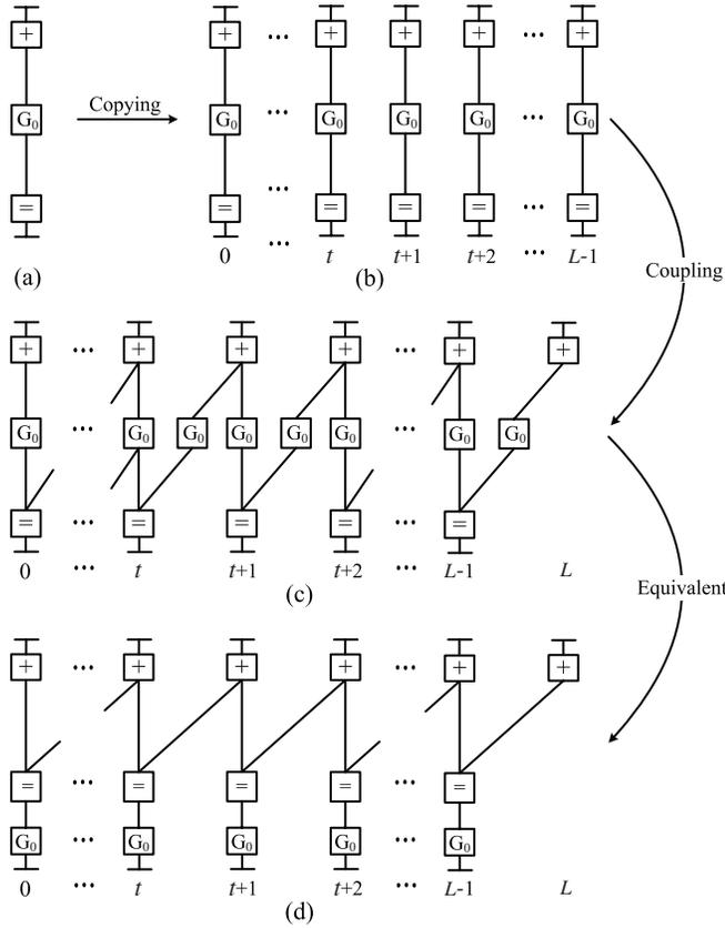
Fig. 4. (a) A protograph representing the basic code with generator matrix  $G_0$ , (b)  $L$  uncoupled basic protographs, each of which corresponds to the generator matrix  $G_0$ , (c) a protograph corresponding to a BMST code ensemble with coupling length  $L$  and coupling width  $m = 1$ , and (d) an equivalent protograph corresponding to the same BMST code ensemble with coupling length  $L$  and coupling width  $m = 1$ .
