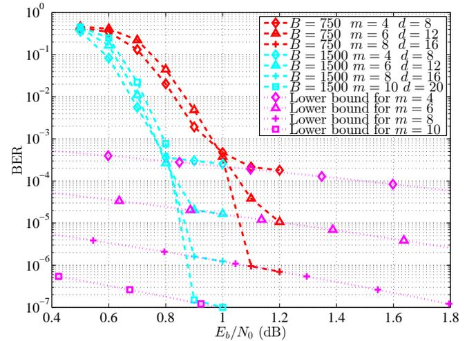
Fig. 10. Simulated decoding performance of rate  $R_{\text{BMST}} = 0.49$  BMST-R [2, 1] codes constructed with different encoding memories  $m$  and decoded with decoding delay  $d = 2m$ . The Cartesian product orders of the involved BMST-R codes are  $B = 750$  and  $B = 1500$ . The corresponding lower bound for BMST-R codes is also plotted.
