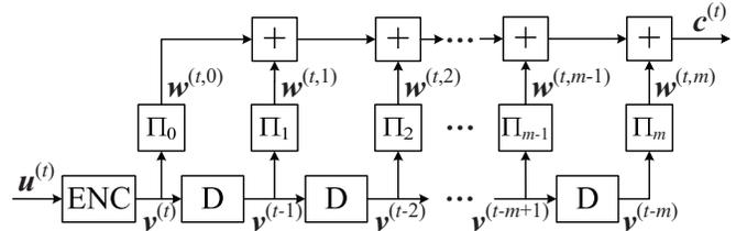
Fig. 1. Encoder of a BMST code with encoding memory  $m$ , where the information sequence  $\mathbf{u}^{(t)}$  at time  $t$  is encoded into the sub-codeword  $\mathbf{c}^{(t)}$  for transmission.
