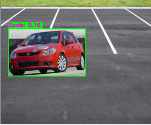
Fig. 4: An example car image placed onto a stationary parking lot background. The scale number annotation corresponds to the ratio of the size of the car compared to the full image.
