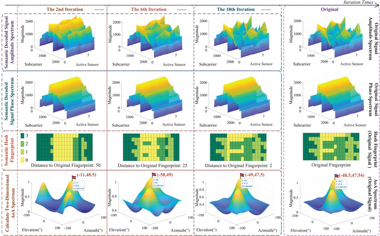
Fig. 6. The variation of the decoded amplitude and phase spectrums at time 4.5 s in the experiment, the corresponding semantic hash matrix, the estimated 2D AoA spectrum by Proposition 2 with the number of outer loop decoding iterations, where the data compression ratio is 5%.
