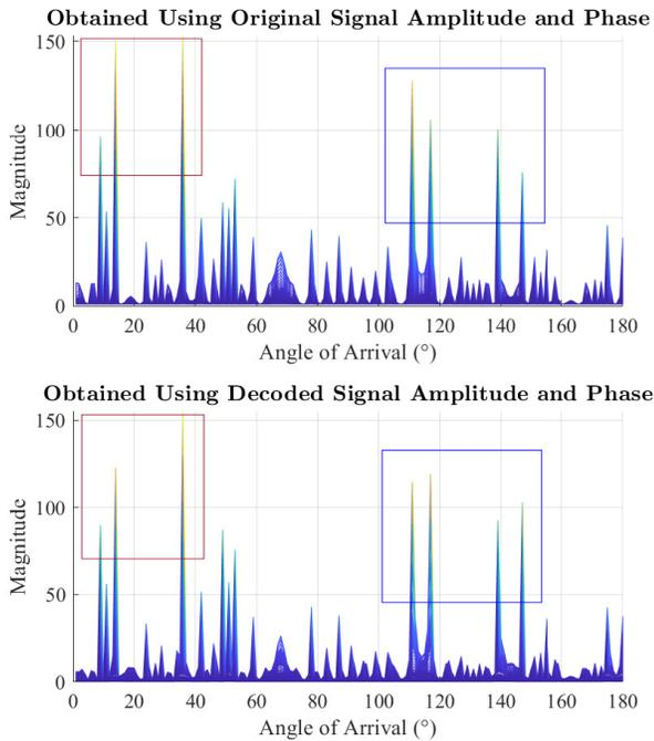
Fig. 9. Comparison of azimuth AoA estimation results that are obtained by using the original and decoded signals, respectively.
