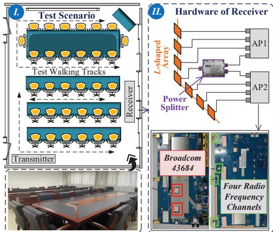
Fig. 5. Test scenario and hardware of the receiver.
