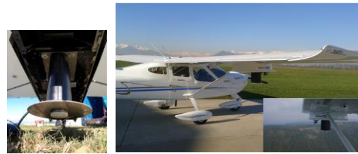
Fig. 3. GNSS-R prototype mounted on Digisky P92 aircraft.
