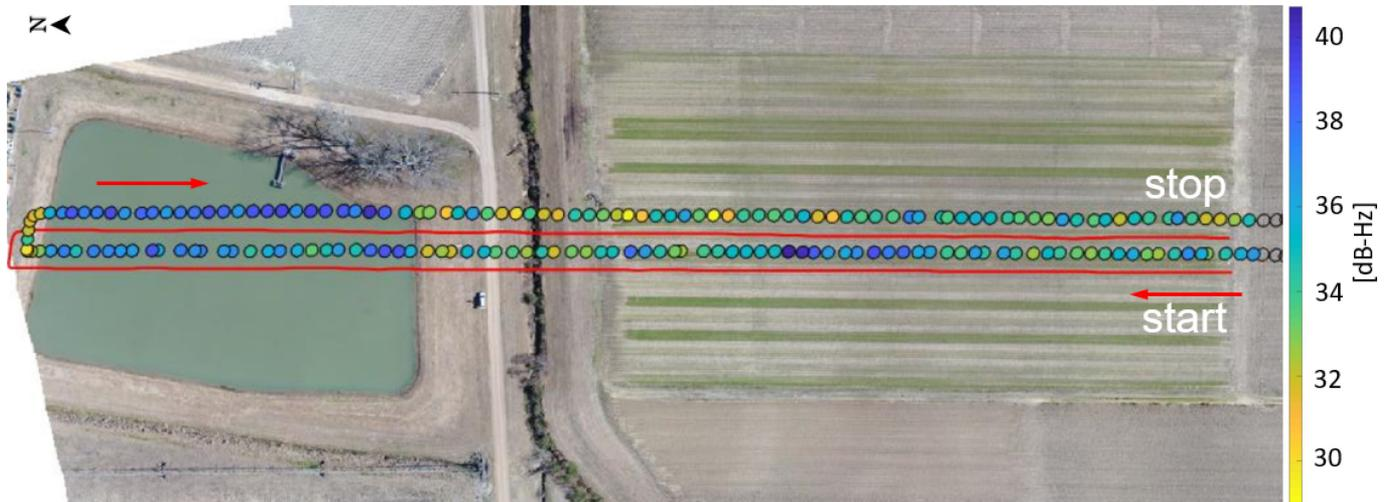
Fig. 10. Flight path (red line) and the smartphone's ground specular reflection tracks associated with PRN #8 satellite are overlaid with the aerial image and colored with  $C/N_0$  (blue being the highest and yellow being the lowest signal strength).
