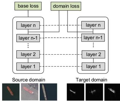
Fig. 4. Illustration of feature-based transfer learning.
