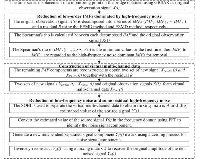
Fig. 1. Flowchart of the proposed de-noising method for the obtained dynamic deflection of bridges using ground-based synthetic aperture radar (GBSAR).
