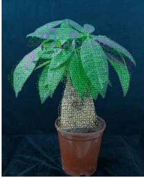
Fig. 12. Registration of HSL point cloud and 2D image.
