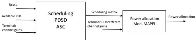
Fig. 1. Simple flowchart of the procedure for NB-IoT resource allocation.
