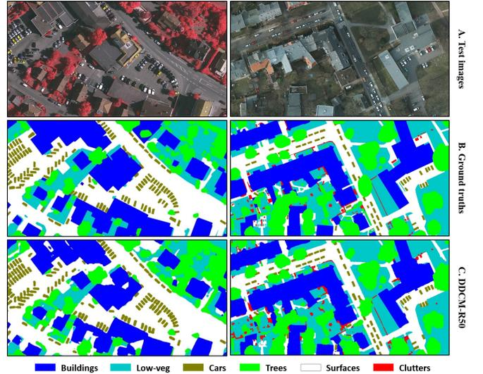
Fig. 4. Mapping results for test images of Vaihingen tile-27 (left) and Potsdam tile-3\_14 (right). A. Test images (top), B. the Ground truths (center), C. DDCM-R50 (bottom).
