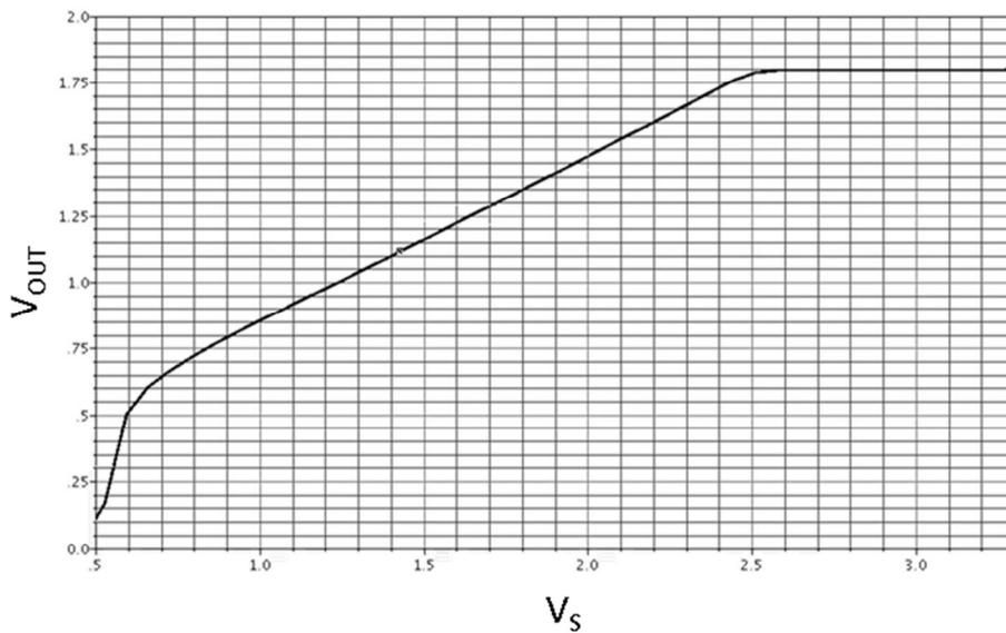
**Figure 47 Input/Output voltage characteristic of LDO**
