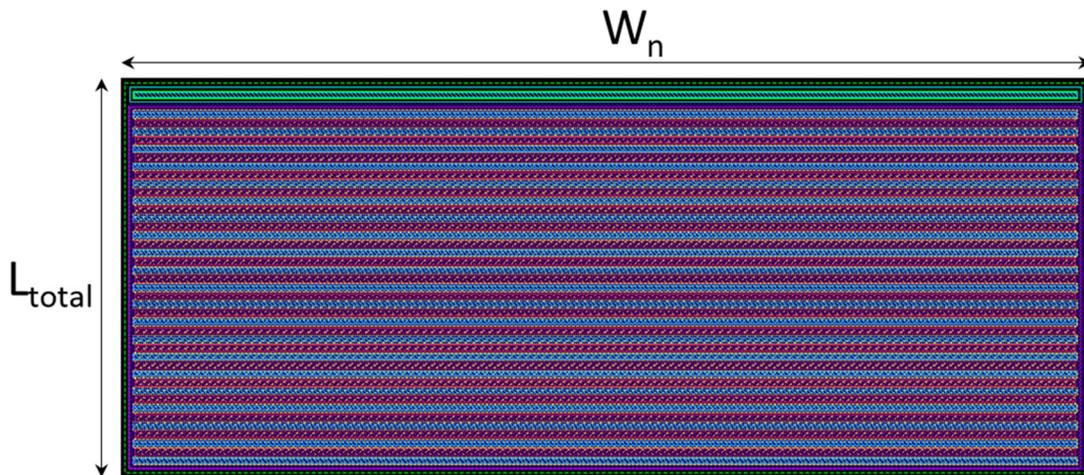
Figure 48 Layout for the 1mm wide PMOS pass transistor
