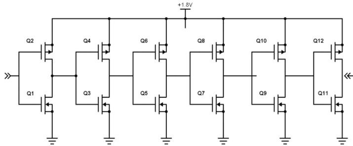
Figure 39 Buffer schematic
