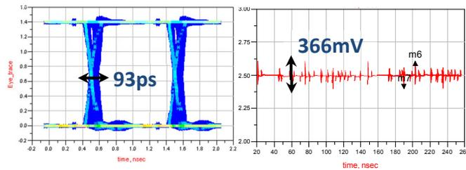
(a) Top layer, jitter = 93ps,  $\Delta V_{DD} = 366\text{mV}$
