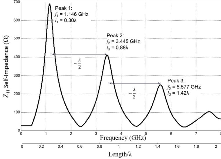
**Figure 88 Simulated  $Z_{11}$  of power transmission line**
