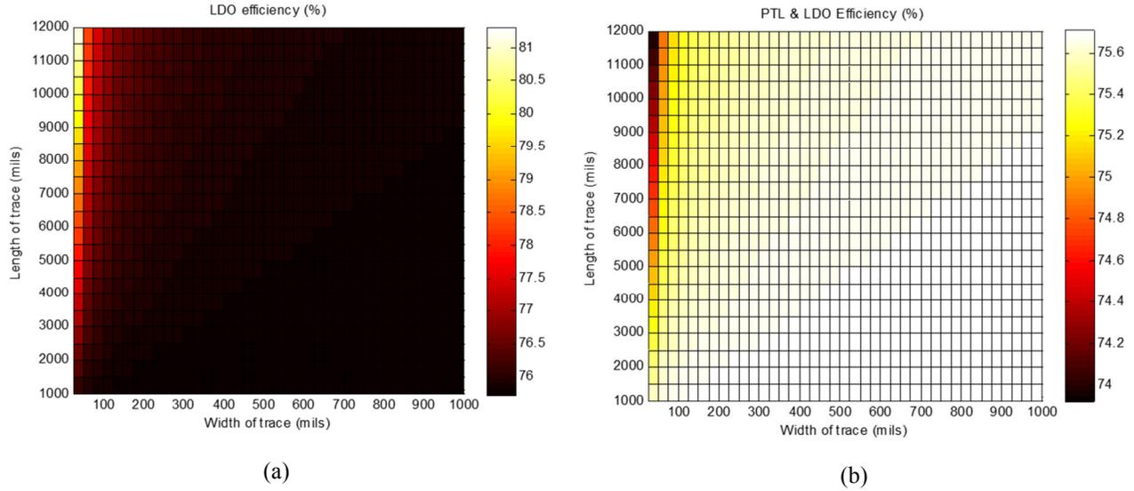
**Figure 102 (a) Power efficiency of the LDO, (b) Power efficiency of the LDO including PTL loss**
