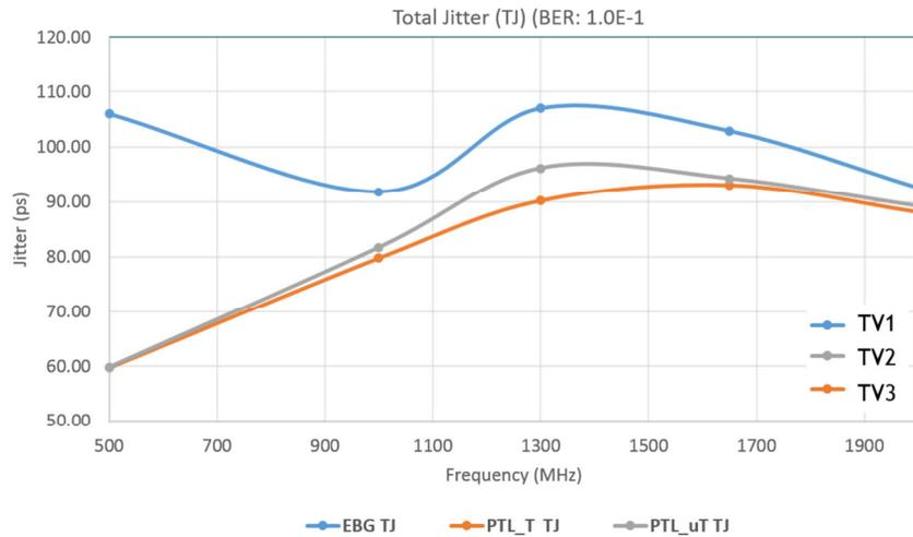
**Figure 91 Total jitter (TJ) measured for all test vehicles**
