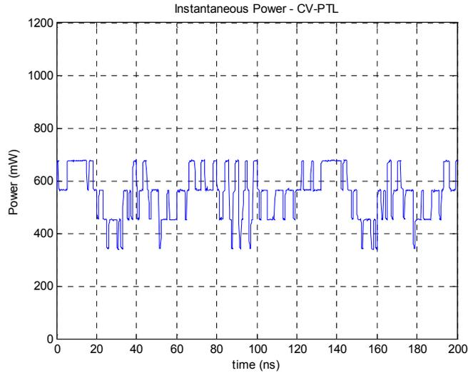
**Figure 26 Instantaneous power consumed by the CV-PTL 3D stack (in mW) with 256-bit long PRBS signal at 1Gbps**
