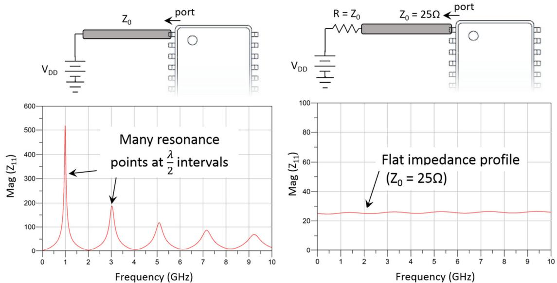
Figure 9 Comparison of PTL's self impedance,  $Z_{11}$ , (left) without termination, (right) with termination
