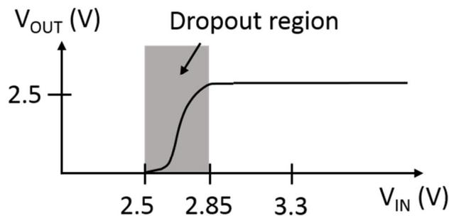
**Figure 103 Dropout voltage of LDO**
