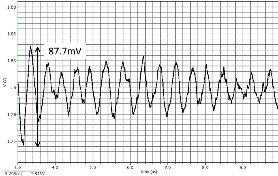
**Figure 43 Power supply noise with 500Mbps PRBS-10 input to all six buffers**
