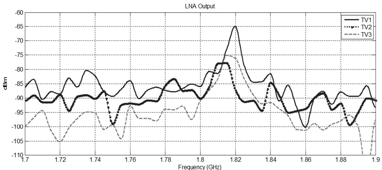
**Figure 95 Frequency domain output of LNA for each test vehicle**
