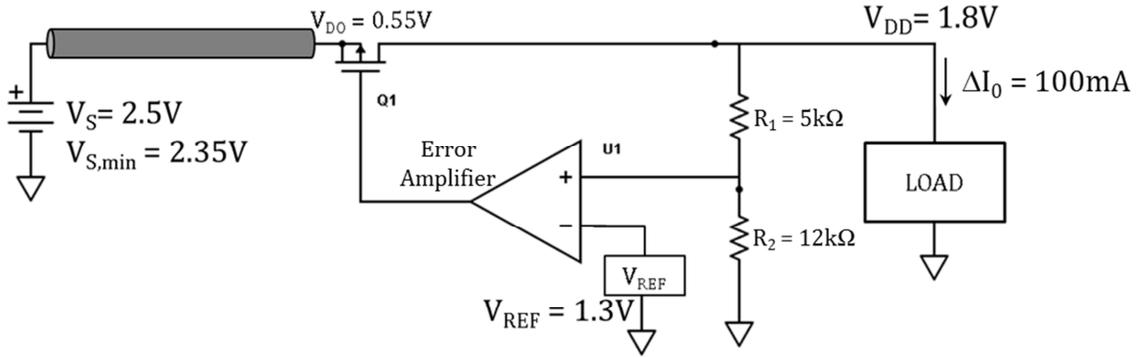
**Figure 29 Voltage regulator circuit schematic**
