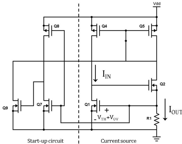
Figure 35 Self-biasing  $V_{th}$  reference circuit with start-up circuit
