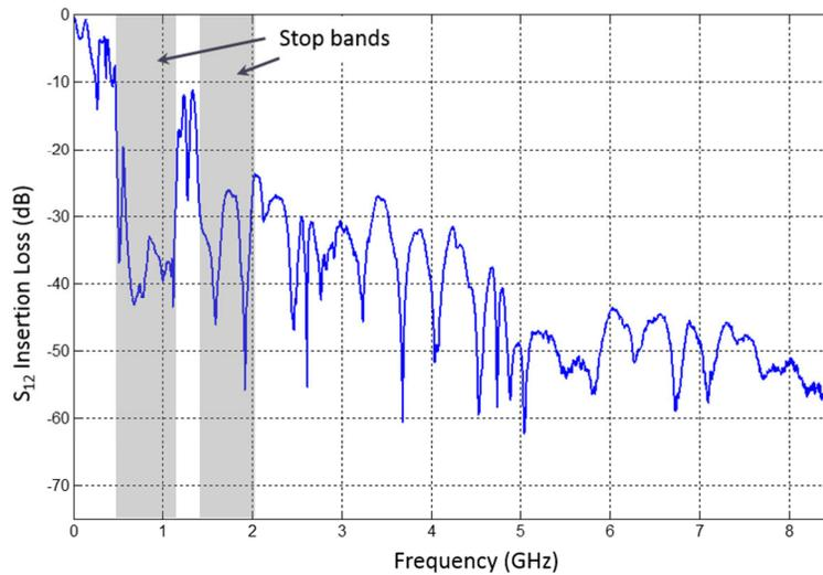
**Figure 77 Electromagnetic band gap measured frequency response**
