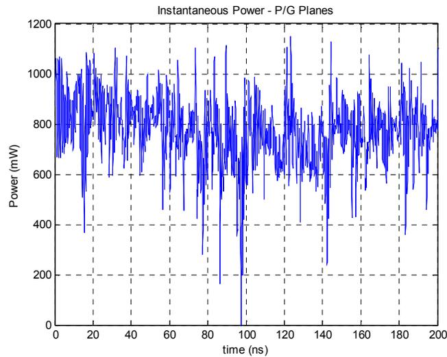
**Figure 27 Instantaneous power consumed by the conventional PDN circuit**
