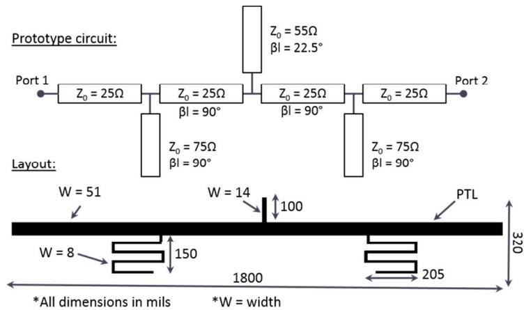
**Figure 82 Layout of microstrip bandstop filter and PTL for TV2**
