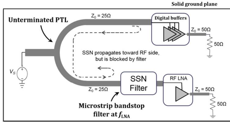
Figure 56 Mixed signal noise isolation concept showing the use of the SSN filter.
