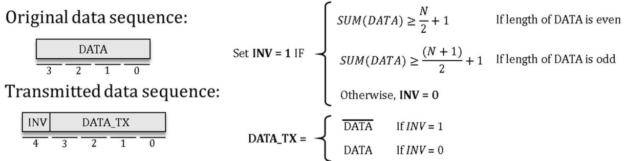
**Figure 14 Bus-inversion encoding scheme**
