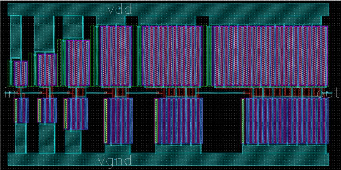
Figure 51 Layout of buffer circuit
