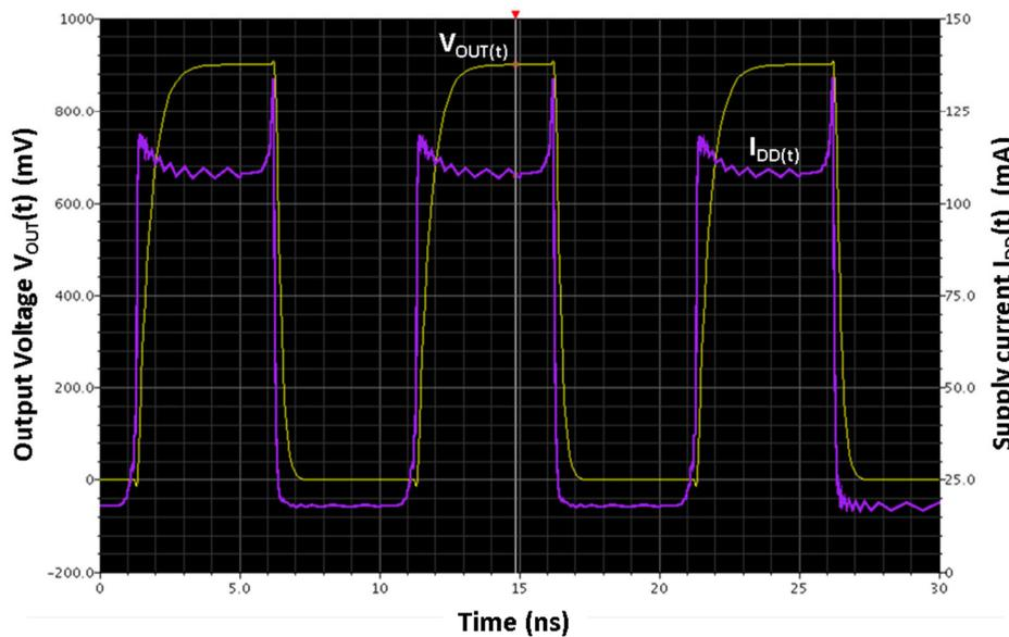
Figure 40 Output voltage of a single buffer and total supply current sourced by all six buffers
