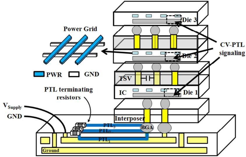
Figure 24 Cross-sectional view of the 3D system using CV-PTL
