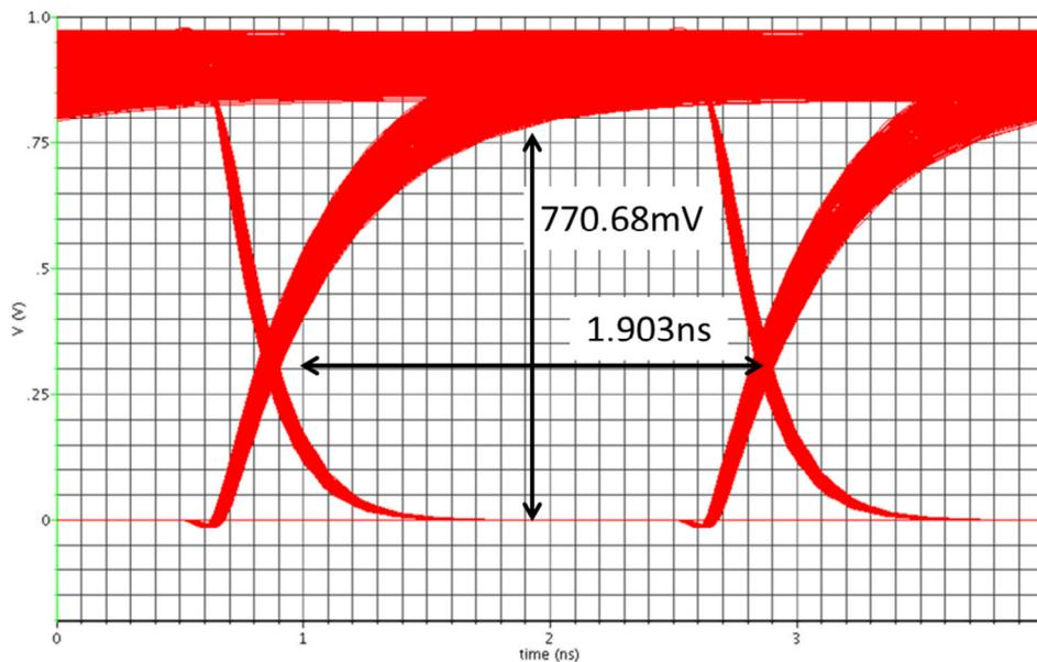
**Figure 45 Eye diagram with 500Mbps PRBS-10 input with LDO powered by power plane**
