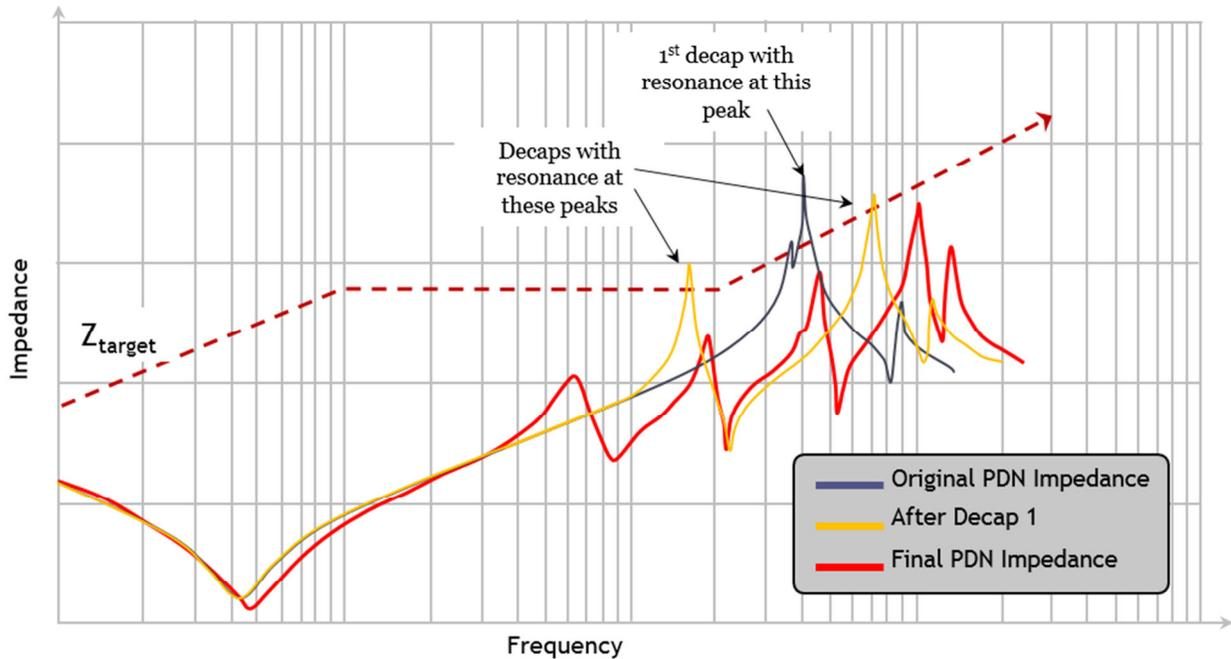
Figure 7 Example of decoupling capacitor placement
