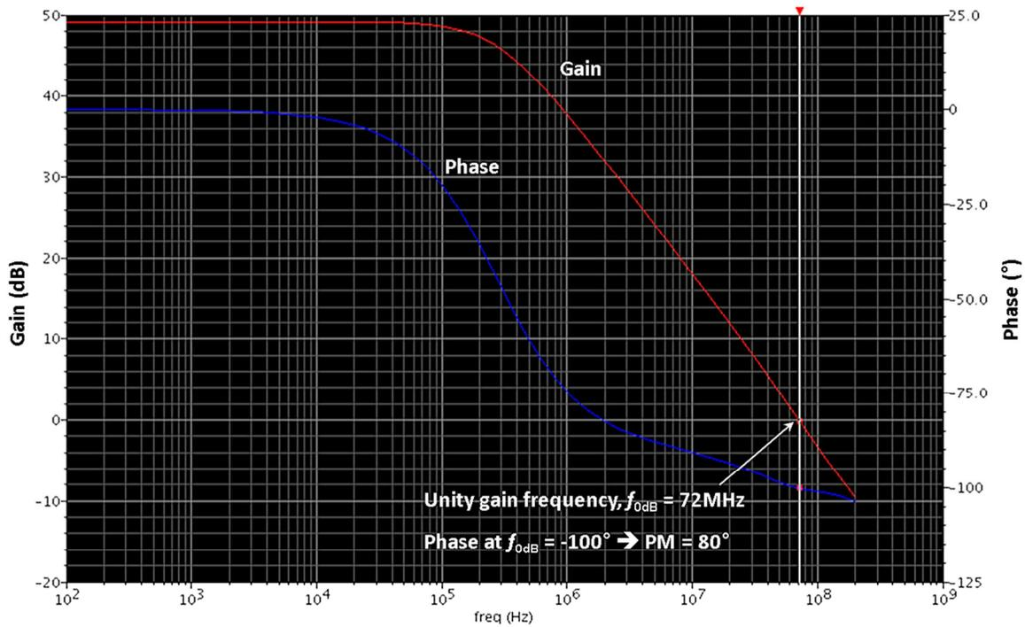
Figure 34 Frequency response of error amplifier
