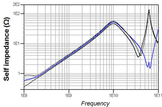
Figure 22 Impedance profile of interposer and stack-up only
