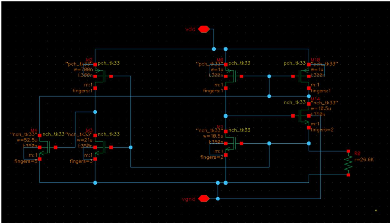
Figure 37 Current reference with start-up circuit
