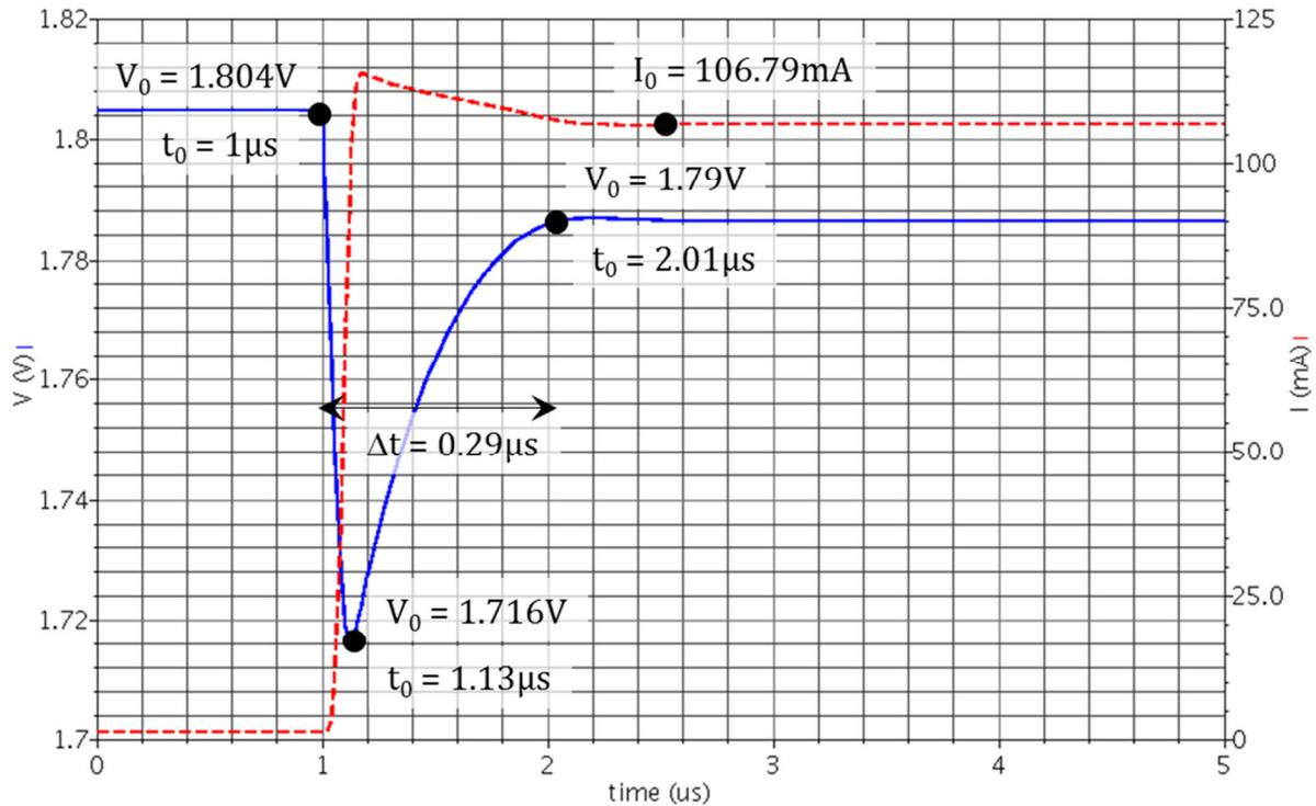
**Figure 41 Output load voltage regulation of LDO corresponding to a 107mA load current step**
