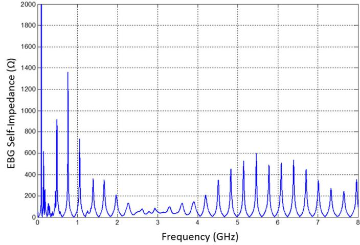
**Figure 78 Measured self-impedance ( $Z_{11}$ ) of EBG structure**
