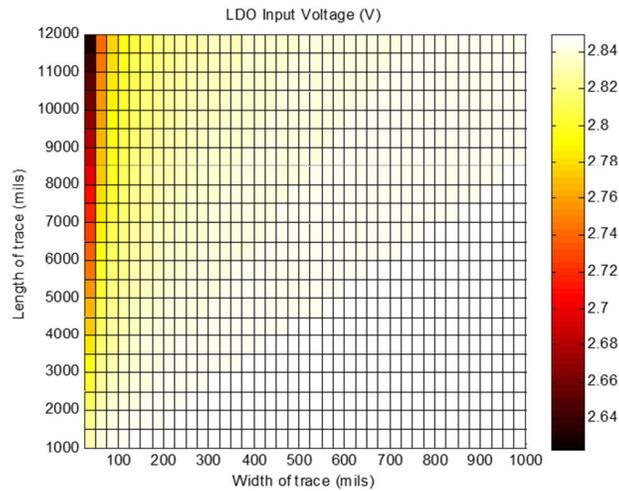
Figure 104 LDO input voltage ( $V_{SW,OUT} = 2.85V$ ,  $V_O = 2.5V$ ,  $I_O = 1A$ )
