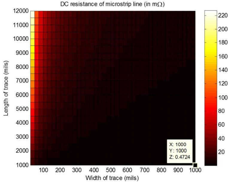
**Figure 100 Total DC resistance (mΩ) for PTL with varying width and length**
