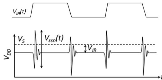
**Figure 4 (top) Input voltage (bottom)  $V_{DD}$  node voltage with ohmic drop and switching noise**
