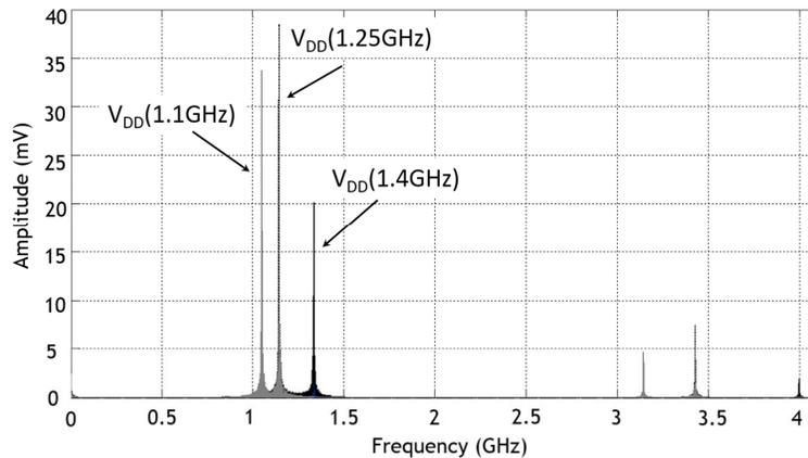
**Figure 89** Calculated  $V_{DD}$  spectrum for three input frequencies
