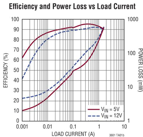
**Figure 97 Efficiency and power loss vs. load current of LTC3601 from Linear Technology [53]**
