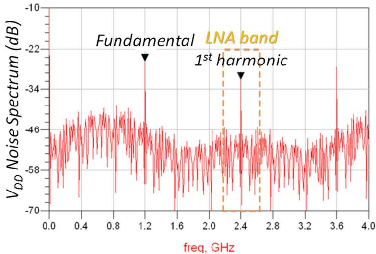
Figure 59 Spectrum of power supply noise
