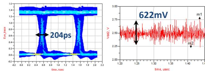
(a) Top layer, jitter = 204ps,  $\Delta V_{DD} = 622\text{mV}$
