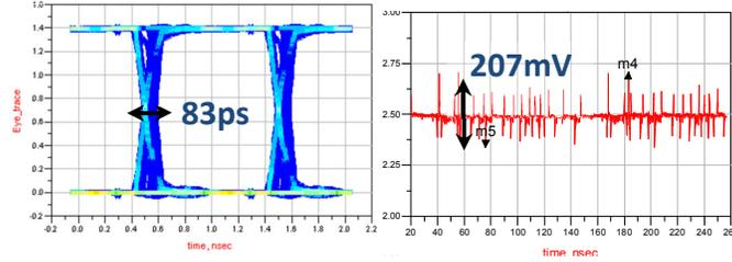
(c) Bottom layer, jitter = 83ps,  $\Delta V_{DD} = 207\text{mV}$
