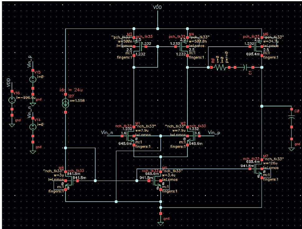
Figure 33 Error amplifier schematic in Cadence
