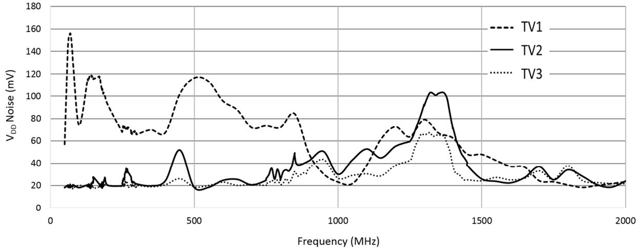
**Figure 87 Measured power supply noise for all test vehicles versus clock frequency**
