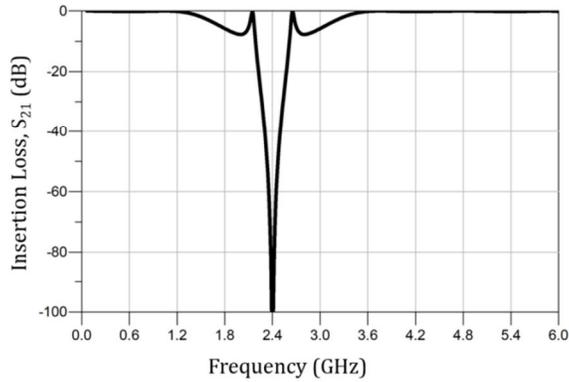
**Figure 64 Frequency response of 2.4GHz bandstop filter**
