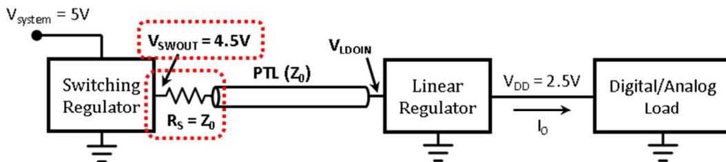
**Figure 107 Power distribution network with a linear regulator powered by a terminated PTL**
