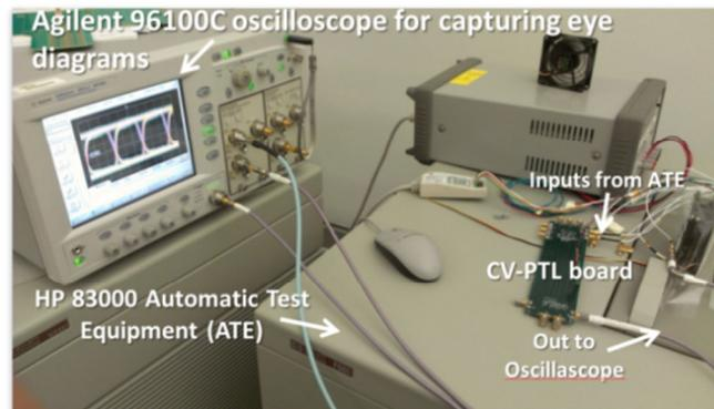
**Figure 17 Laboratory setup for measurements**
