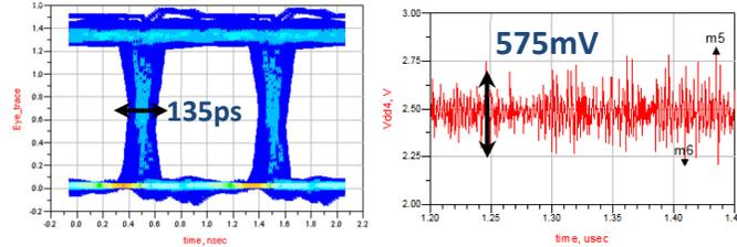
(c) Bottom layer, jitter = 135ps,  $\Delta V_{DD} = 575\text{mV}$
