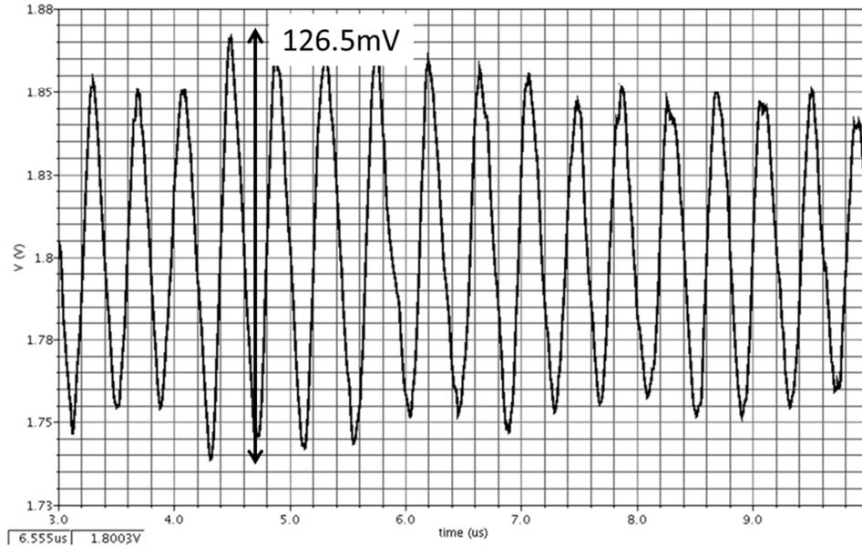
**Figure 46 Power supply noise with 500Mbps PRBS-10 input to all six buffers**
