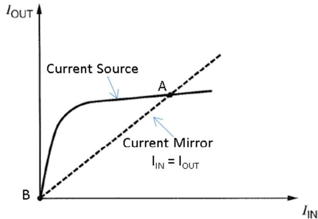
Figure 36 Operating point of self-biased reference circuit (reproduced from [33])
