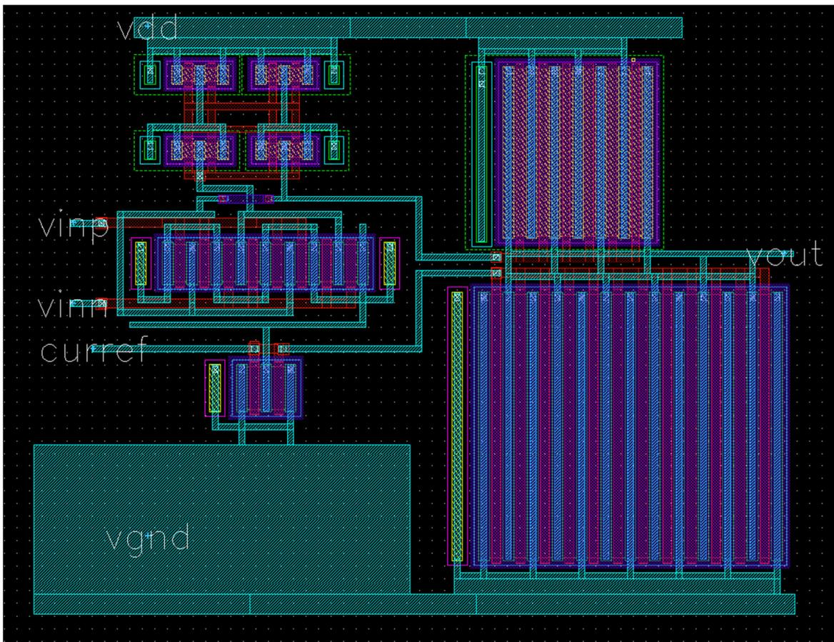
Figure 49 Layout of error amplifier (without current reference circuit)
