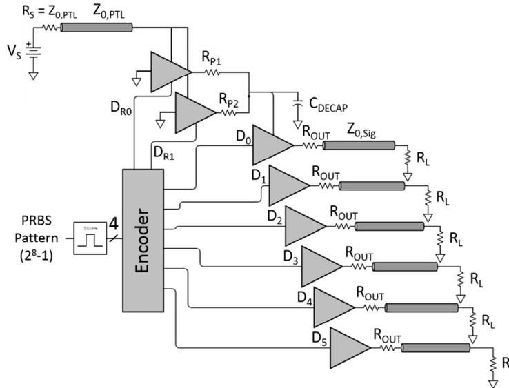
**Figure 13 Constant Voltage Power Transmission Line topology as implemented on test vehicle**
