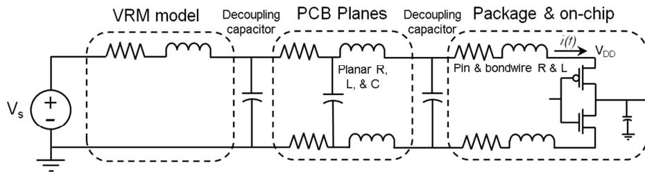
**Figure 2 Simplified circuit schematic of a standard power distribution network**
