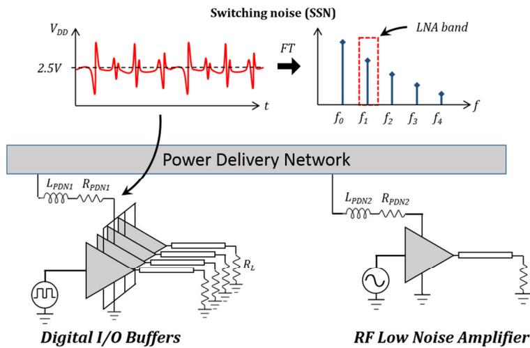
Figure 55 Power supply noise coupling
