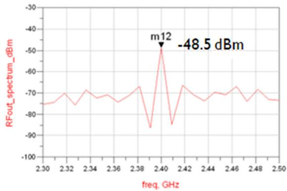
Figure 63 LNA output spectrum at 2.4 GHz
