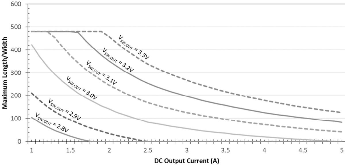
**Figure 106 Design curves for maximum PTL (W/L) to support a specified DC output current**
