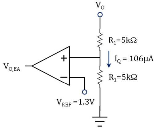
Figure 38 Voltage divider used for output sampling
