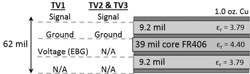
**Figure 79 Test vehicle cross-section**
