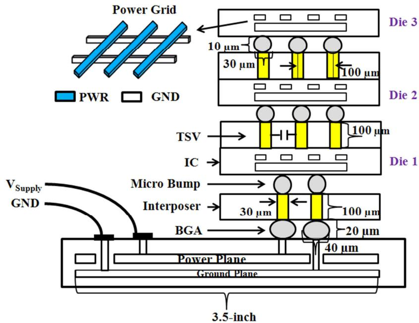
Figure 20 Cross-sectional view of a conventional power-plane 3D system [8, 19]
