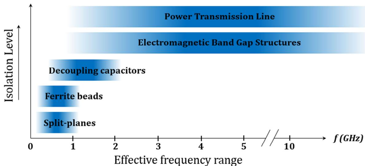
Figure 53 Effective frequency range of several noise isolation techniques
