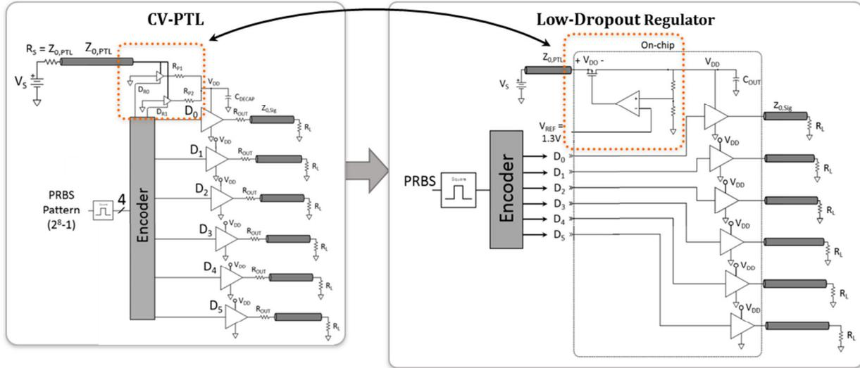
**Figure 28 Schematic of CV-PTL implementation and voltage regulator circuit**
