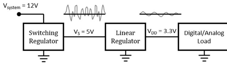
Figure 96 Power distribution with a switching and linear regulator
