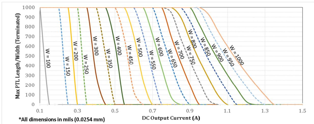
**Figure 108 Design curves for maximum PTL (W/L) to support a specified DC output current when using a terminated PTL**
