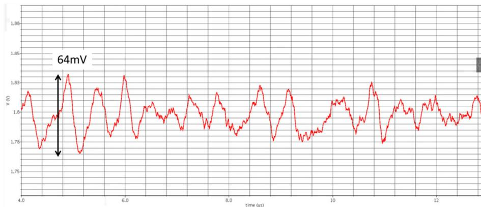
**Figure 44 Power supply noise with terminated PTL**
