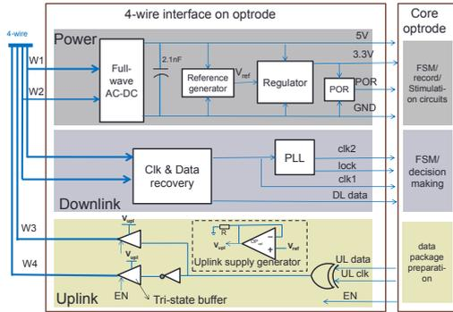
Fig. 2: Top-level system architecture for the 4-wire interface.
