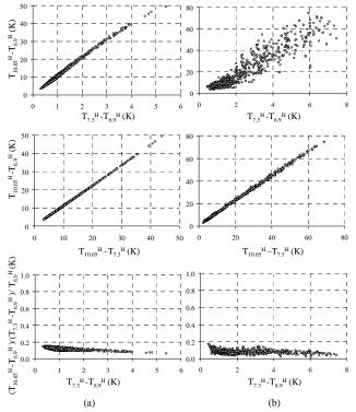
Fig. 1. Spectral difference functions of AMSR2 measurements at horizontal polarization at C- and X-band channels for natural atmospheric and oceanic parameter variations: (a) model calculations without precipitation; (b) AMSR2 measurements over the oceans, including precipitating areas.
