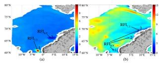
Fig. 3. AMSR2 spectral differences on 1 January 2012 at ~ 11:18 UTC: (a)  $T_{7.3}^{-1}$  -  $T_{6.9}^{-H}$  (K); (b)  $T_{10.65}^{-H}$  -  $T_{6.9}^{-H}$  (K).
