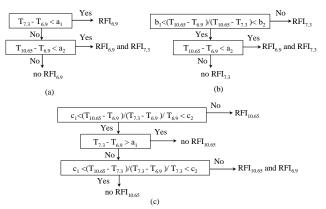
Fig. 2. Decision tree for identification RFI contaminated pixels: (a) at 6.9 GHz; (b) at 7.3 GHz; (c) at 10.65 GHz. For horizontally polarized radiation  $a_1=0.3K$ ,  $a_2=3.3K$ ,  $b_1=1.07$ ,  $b_2=1.4$ ,  $c_1=0.03K^{-1}$ ,  $c_2=0.15K^{-1}$ . For vertically polarized radiation  $a_1=0.3K$ ,  $a_2=3.6K$ ,  $b_1=1.04$ ,  $b_2=1.1$ ,  $c_1=0.03K^{-1}$ ,  $c_2=0.15K^{-1}$ .
