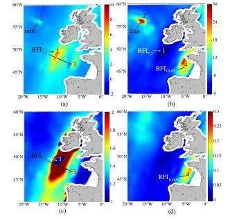
Fig. 4. AMSR2 measurement data on 3 September 2012 at ~ 03:23 UTC: (a)  $T_{7,3}^{H}-T_{6,9}^{H}$  (K); (b)  $T_{10,65}^{H}-T_{7,3}^{H}$  (K); (c)  $DT_{X,C1}/DT_{C2,C1}$  (dimensionless unit); (d)  $DT_{X,C2}/DT_{C1,C2}/T_{C2}$  (K<sup>-1</sup>).
