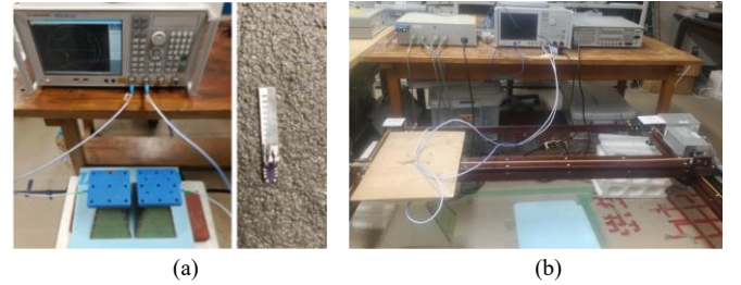
Fig. 10. Experiment setups. (a) Temperature change monitoring; (b) Synthetic aperture measurement.
