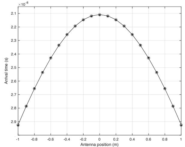
Fig. 3. Three almost identical hyperbolas with different  $\{d, R, \epsilon\}$  are plotted together to illustrate the non-unique results of hyperbola fitting in the presence of noise. Solid line:  $d = 1$  m,  $R = 0.1$  m,  $\epsilon_r = 10$ ; circles:  $d = 0.97$  m,  $R = 0.2$  m,  $\epsilon_r = 10.6$ ; stars:  $d = 0.91$  m,  $R = 0.4$  m,  $\epsilon_r = 12.1$ .
