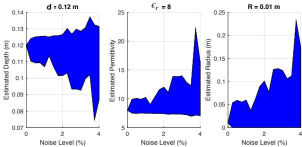
Fig. 4. Concrete inspection: 120 realisations of hyperbola fitting (4) for different sets of Gaussian noise in each execution. The real  $\{d, R, \epsilon_r\}$  are shown on the titles of the subplots. The error for  $R$  can go up to 500% with less than 2% of noise level, falsely estimating the radius of the rebar anywhere from 0 up to 0.06 m. This range includes the whole spectrum of rebar sizes, adding no additional information to what is already expected.
