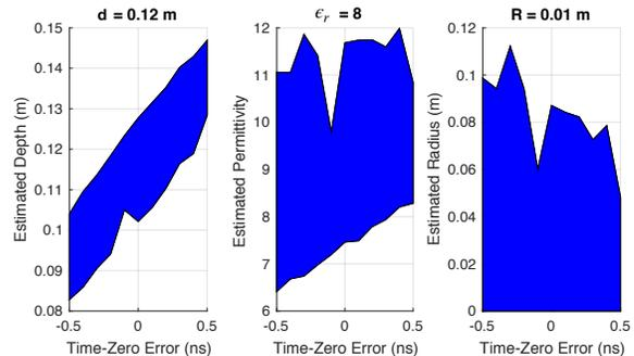
Fig. 6. The effect of time-zero error to the estimated  $\{d, R, \epsilon_r\}$ . The noise level is 1% for all the experiments. With blue colour is the range of  $\{d, R, \epsilon_r\}$  that equally fits the arrival times. The real  $\{d, R, \epsilon_r\}$  are shown on the titles of the subplots.
