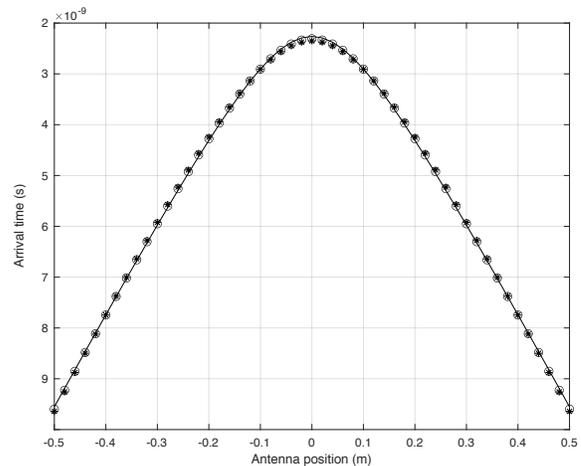
Fig. 5. Three almost identical hyperbolas with different  $\{d, R, \epsilon_r\}$  are plotted together to illustrate the non-unique results of hyperbola fitting in the presence of noise. Solid line:  $d = 0.12$  m,  $R = 0.01$  m,  $\epsilon_r = 8$ ; circles:  $d = 0.118$  m,  $R = 0.03$  m,  $\epsilon_r = 8.5$ ; stars:  $d = 0.116$  m,  $R = 0.05$  m,  $\epsilon_r = 9.1$ .
