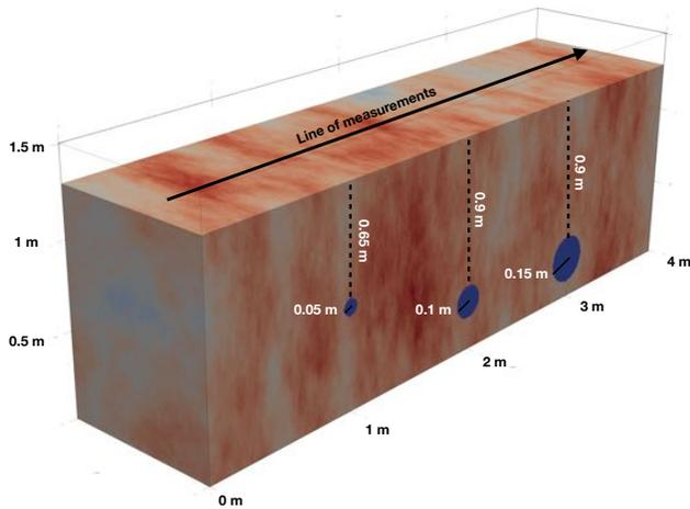
Fig. 7. The investigated numerical study. Three homogeneous low-dielectric ( $\epsilon_r = 3$ ) pipes with different radii  $R = [0.05, 0.1, 0.15]$  m, are buried in a stochastic medium with varying water fraction from 2-10% ( $\epsilon_r \approx 4 - 9$ ). Red and light blue colours correspond to dry and saturated areas, respectively.
