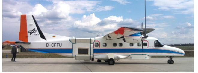
Fig. 1. DLR aircraft Dornier Do228-212, with mounted F-SAR antenna carrier (middle-end part of the fuselage).
