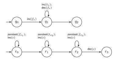
Fig. 5. Reduction for CMs. The top gadget shows variable assignment. The bottom gadget shows the checks for a clause  $c \equiv x_1 \lor \neg x_2 \lor x_3$ .
