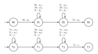
Fig. 6. Reduction for CFSMs. The top gadget shows variable selection. The bottom gadget shows the checks for a clause  $x_1 \lor \neg x_2 \lor x_3$ .
