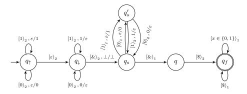
Fig. 1. 2-HPDA accepting  $\{w\&w \mid w \in (\{0,1\})^* \text{ and } w \text{ is a palindrome}\}, \perp \text{ is the end-of-stack symbol}$
