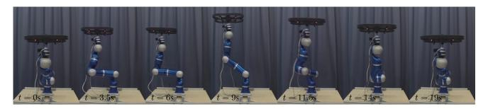
Fig. 7. Picture sequence from the experiment with the controller from Section III-C, the indicated time instants correspond to the plot in Fig. 10. A short video by the authors of this paper showing the VTOL UAV landing system demonstrator and some of the conducted experiments is provided online [18].
