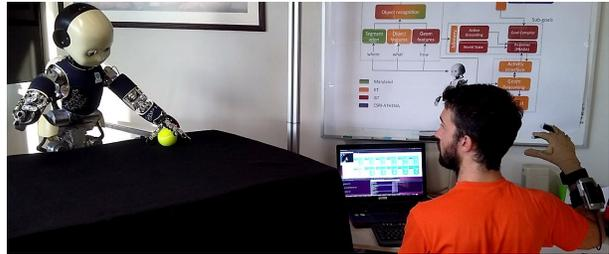
Fig. 1. Experimental setup. The fingers of the iCub robot hand (on the left) are controlled by a human operator with the CyberGlove-II dataglove (on the right).
