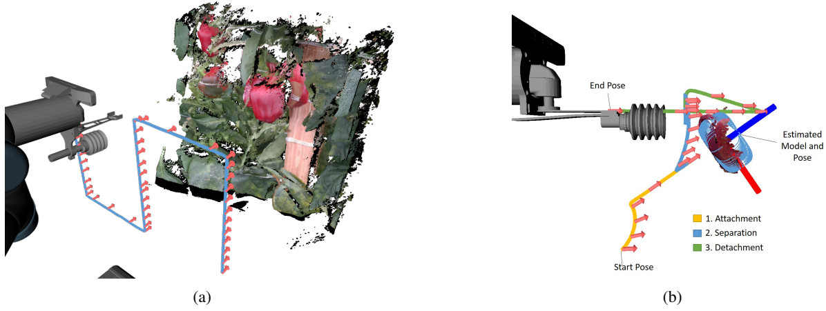
Fig. 6: (a) Scanning trajectory of the camera during a single field trial along with the registered point cloud (b) End effector trajectory of a single harvesting trial. The end effector position and orientation is indicated by a coloured line and red arrow, respectively. The trajectory begins (start pose) with the attachment stage (yellow line), transitioning into the separation stage (blue line) and finishing with the detachment stage (green line). The estimated pose of the sweet pepper is shown using blue and red axes.
