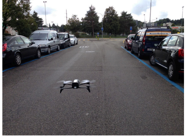
Fig. 1: DroNet is a convolutional neural network, whose purpose is to reliably drive an autonomous drone through the streets of a city. Trained with data collected by cars and bicycles, our system learns from them to follow basic traffic rules, e.g. do not go out of the road, and to safely avoid other pedestrians or obstacles. Surprisingly, the policy learned by DroNet is highly generalizable, and even allows to fly a drone on indoor corridors and parking lots.
