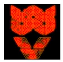
Fig. 5: Map of skin response while the skin is being calibrated. The brightness of the red color indicates the change in capacitance value. It can be seen that the sensors have different responses to the uniform applied pressure.
