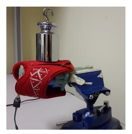
Fig. 9: Validation setup. Different masses with known weights were placed on the skin. A level was used to ensure the weight vector is normal to the ground.
