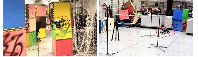
(a) Fast autonomous flight in an unknown environment. (b) Aggressive kinodynamic replanning with indoor external feedback.
