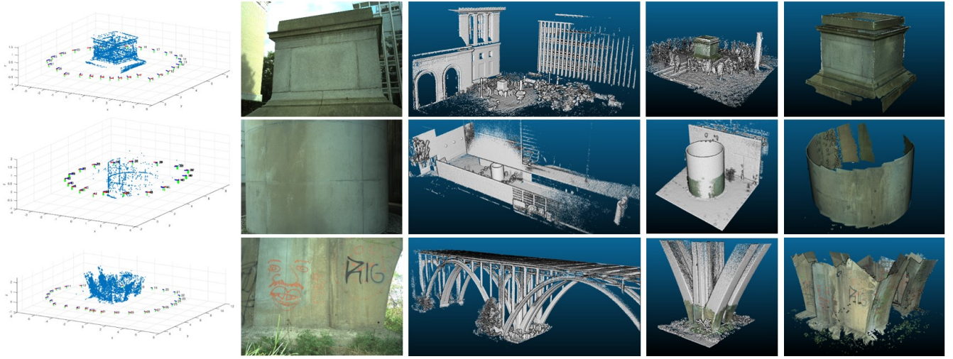
Fig. 9: From top to bottom, the results of three tests are visualized: a squared pillar (top), a cylinder pillar (middle) and a bridge pillar (bottom). From left to right, we visualize the camera poses and landmarks (blue points), a sample of the image data, complete LiDAR point cloud, overlaid LiDAR and stereo point cloud, dense stereo point cloud.
