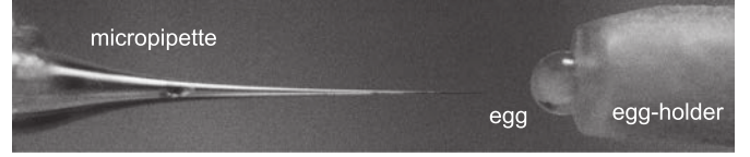
Fig. 5. Micropipette and egg holder. The pipette had a diameter of \sim 10 \mu\text{m} and egg specimens were immobilised by suction.
