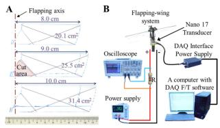
Fig. 4. Experimental setup. (A) Wings with different wing areas at the same aspect ratio of 3.2. (B) Experimental apparatus for force and power measurements.
