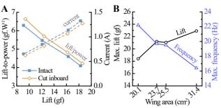
Fig. 8. (A) Effect of wing inboard area on lift-to-power ratio. (B) Maximum lift and frequency powered by a single lithium polymer battery (3.7V) for different wing areas at an amplitude of about 190°. Maximum force SD =  $\pm 0.2$  gf).
