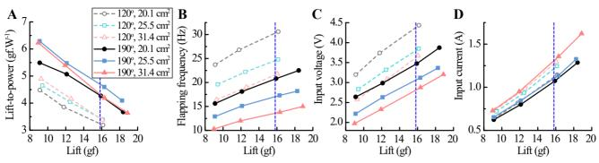
Fig. 5. Generation of lift or vertical force at different stroke amplitudes and wing areas. (A) Lift-to-power with respect to lift generation. (B) Lift versus flapping frequency (C) Lift versus input voltage. (D) Lift versus input current. Vertical dashed-blue line represents the body weight of the robot. Maximum force SD =  $\pm 0.2$  gram force (gf). (1.0 gf = 9.8 mN).
