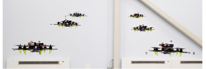
Fig. 1. Six multirotors in a slanted plane formation. Vehicles communicate with each other, make distributed decisions onboard, and use VIO for localization.
