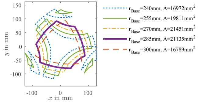
Fig. 4. Workspace contours for various values of the base radius  $r_{Base}$ . The  $0^\circ$  translational workspace of the PCR was obtained by discretizing the joint space and intersecting the leg workspaces which result from applying alpha shapes to the discretized point clouds.
