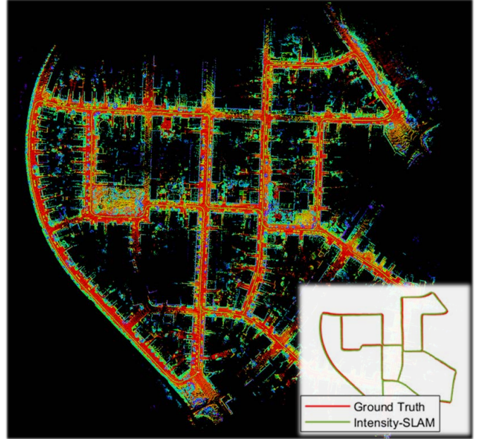
Fig. 1: Example of localization and mapping from the proposed method on KITTI sequence 00. The localization result is shown on the right corner with the ground truth plotted in red color and the trajectory plotted in green color. Our method achieves much higher localization accuracy compared to geometric-only methods.
