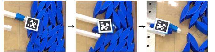
Fig. 4: Dig-grasping for planar bin picking: align (left) - dig (middle) - pinch (right). The marked object instance is being dig-grasped from the clutter.
