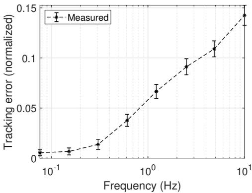
Fig. 10. **The results of the tracking of a sinusoidal reference input:** We conduct the trajectory tracking experiment by changing the frequency of the sinusoidal reference trajectory. We show RMS tracking error at different frequencies.
