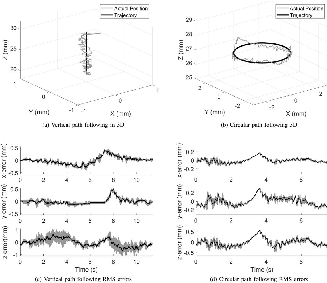
Fig. 9. **Trajectory tracking experiment results:** In these tests, the module follows a vertical straight line and a circular path. We compare 3D target trajectories and actual module end-effector positions in (a) and (b). Furthermore, we provide RMS tracking errors with shaded error regions in cartesian coordinates in (c) and (d).
