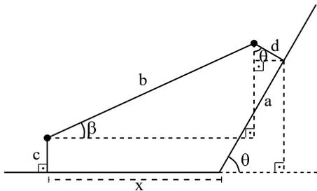
Fig. 3. Sensor kinematic model in 2D
