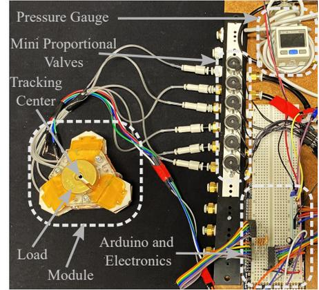
Fig. 8. **Experimental setup for pneumatic control:** the setup consists of six miniature proportional valves, a pressure gauge, an Arduino board, electronic components, flexible tubes, a load, and the module.
