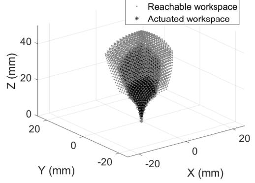
Fig. 7. **Current pneumagami module prototype workspace using forward kinematic model:** The plot shows the reachable workspace of the module without any actuator and achievable workspace with pouch motors. The workspace with actuator is limited since we can achieve 0 to 60°s folding at the legs with the pouch motors, whereas the structure design allows 0-90°s folding angle.
