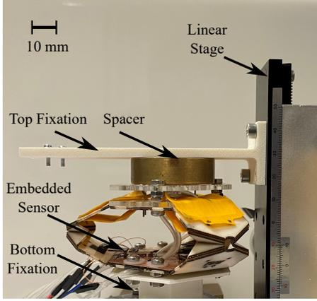
Fig. 4. **Sensor characterization:** We attach the module end effector to a linear stage using a spacer and a fixation. While keeping the module's top and bottom hexagons parallel, we increase the module's height by 5 mm steps by changing the position of the end effector manually. Then, we record the actual height and sensory data. Finally, using sensor kinematics, we calculate the leg angle.
