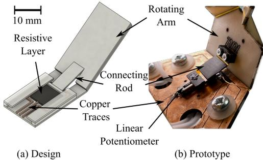
Fig. 2. **Embedded sensor mechanism and design:** We place an origami slider connected to the rotating arm on copper and resistive layers. When the arm rotates, the slider mechanism converts rotational motion into one DoF translational motion. The slider moves on the resistive layer and changes the measured resistance. By utilizing the kinematics of the transmission, we measure the folding angle.
