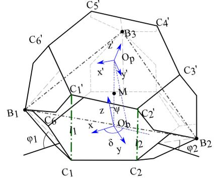
Fig. 6. Kinematic model of parallel pneumagami module and model parameters
