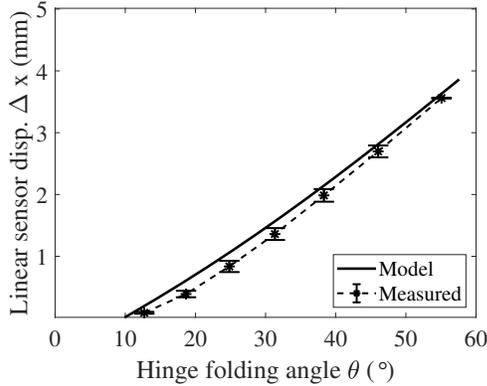
Fig. 5. **Model vs measured folding angle:** We repeat the experiment four times and plot the average measured data with error bars. Then, we compare it with the model. The RMS error between the model and measured data is around 2.2°.
