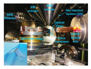
Fig. 3. Experimental configuration for welding and activating the polyarticulated origami structures with a stretched optical fiber tip. The locally zoomed-in rendering at the bottom left shows the micro origami structure folded on the silica membrane.
