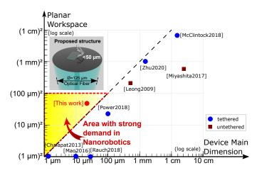
Fig. 1. Comparison of the device size and approximate planar workspace of some representative active origami robots and micro structures developed in recent years. The devices in the area above the dotted line indicate that they have a large workspace compared to their size. Among them, large workspace sub-100  $\mu$ m devices are in high demand for the development of nanorobotics [3], [15], [16].
