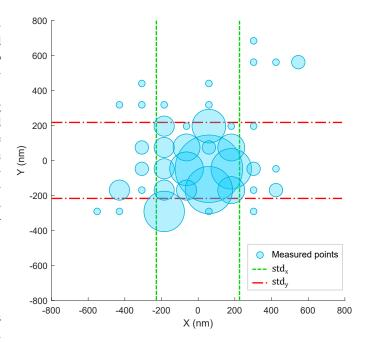
Fig. 8. Repeatability test, distribution of the results of 100 measurements for 20 repetitions of the determined pose (5 measurements per pose), The size of bubble indicates the density of the data measured at that point.
