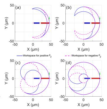
Fig. 4. Workspace simulation results obtained using analytical method, for different joint limits of  $\theta_1$  and  $\theta_2$ . (a)  $-60^\circ \le \theta_1, \theta_2 \le 60^\circ$ , (b)  $-90^\circ \le \theta_1, \theta_2 \le 90^\circ$ , (c)  $-120^\circ \le \theta_1, \theta_2 \le 120^\circ$ , (d)  $-150^\circ \le \theta_1, \theta_2 \le 150^\circ$ .
