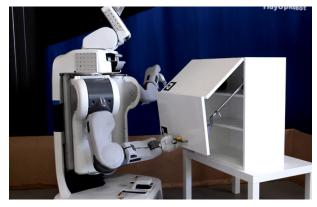
Fig. 7: PR2 operating real folding door kinematic during our experiments.
