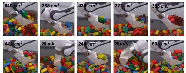
**Fig. 10:** The two rows of images show two excavation episodes for RL-rep-exv in the real world. We also label the bucket filling volume (if not stuck).
