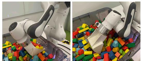
**Fig. 11:** Two typical failure cases of excavation planning due to collision with the tray are shown in the figure. The collisions in the left and right images happen during the closing and dragging phases respectively.
