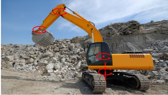
**Fig. 1:** The figure shows an excavator excavating fragmented rocks, with joints labeled in red. An excavator has a total of 4 degrees of freedom, excluding the mobile base.
