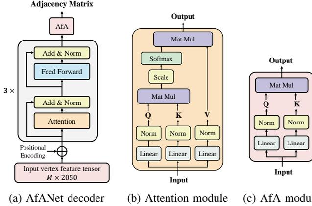
Fig. 6: The visualization of AfANet decoder. Taken  $M \times 2050$ -sized vertex embedding tensor as input, AfANet decoder predicts the  $M \times M$ -sized adjacency matrix of extracted graph vertices. (a) The general network structure of the AfANet decoder; (b) The modified attention module; (c) The Afa module.
