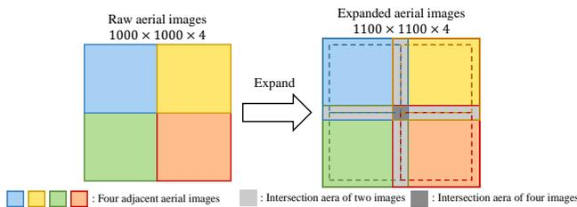
Fig. 3: Visualization of image patch expansion. In this paper, all aerial image patches are expanded into  $1100 \times 1100$ -size, which creates intersection areas between adjacent patches (light gray and dark gray areas). Dashed rectangles on the right represent the original image edges. These intersection areas will benefit the graph stitching process.
