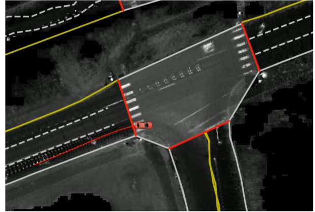
Fig. 1. An online HD map overlaying lidar intensity as a vehicle traverses an intersection. The white and yellow lines indicate inferred road and lane boundaries while the red lines denote intersection entry/exit ports. The background shows a projection of the lidar intensity data into the birds-eye-view (BEV) that was used to help generate the HD map online.
