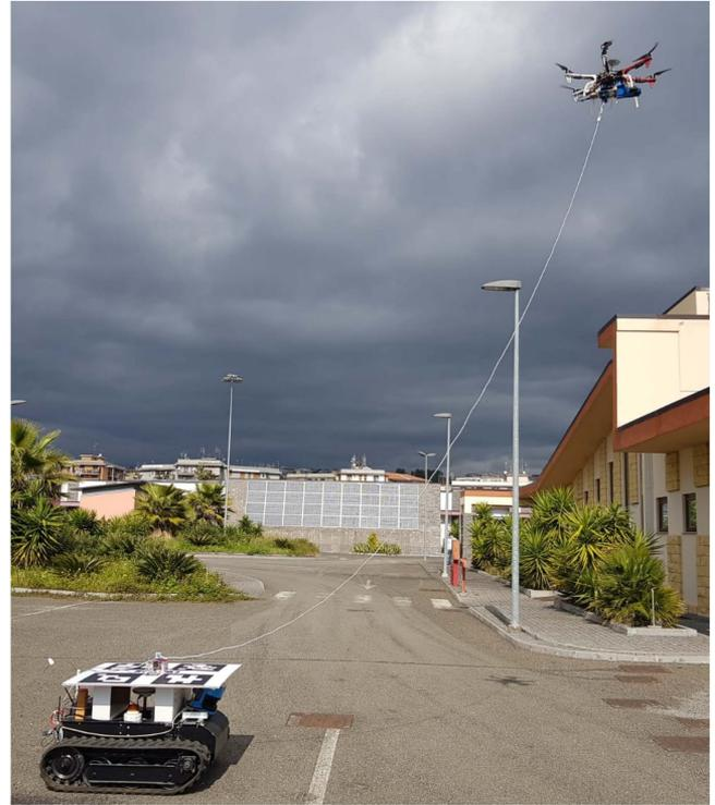
Fig. 7. The multi-robot tethered system with the cable in catenary configuration during operation.
