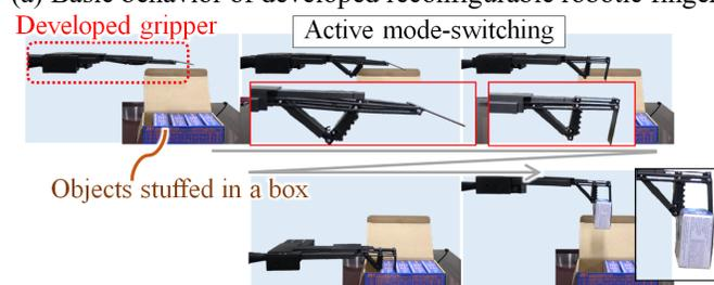
(b) Picking an object stuffed in a box using active switching
