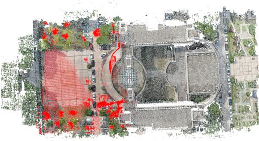
Fig. 3. GNSS Registration, red one is LiDAR-based point cloud, others are the vision-based point cloud. There is an obvious mismatch in the cylindrical tower.
