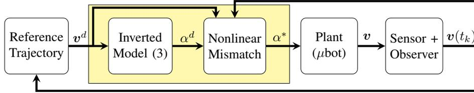
Fig. 3. A control block diagram showing how our proposed system (yellow box) transforms the desired velocity signal ( $v^d$ ) into a heading angle ( $\alpha^*$ ) such that the difference between  $v^d$  and  $v$  is minimized.
