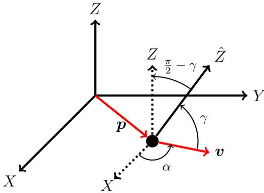
Fig. 2. Schematic illustrating the notation. The solid axes  $X, Y, Z$  define the Cartesian coordinate system. The motion of the  $\mu$ bot is in the  $(X, Y)$  - plane. The fixed attitude angle  $\gamma$  is out of the plane, while the heading angle  $\alpha$  is in plane. The frequency  $f$  determines the  $\mu$ bot's forward speed along  $\mathbf{v}$ , which is in the  $(X, Y)$  - plane.
