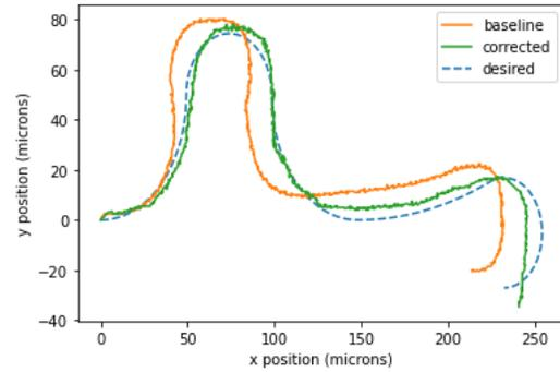
Fig. 7. A comparison of the baseline (orange), corrected (green), and desired (blue, dashed) trajectories from the *in situ* experiment.
