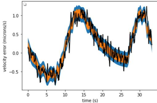
Fig. 5. The GP’s prediction of the  $x$ -axis velocity errors at each time step; the orange band corresponds to one standard deviation (65%), and the blue band corresponds to two standard deviations (95%) of uncertainty. The black line is the actual velocity error.
