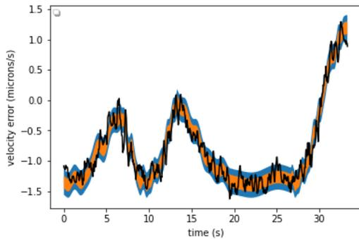
Fig. 6. The GP’s prediction of the  $y$ -axis velocity errors at each time step; orange band corresponds to one standard deviation (65%), and the blue band corresponds to two standard deviations (95%) of uncertainty. The black line is the actual velocity error.
