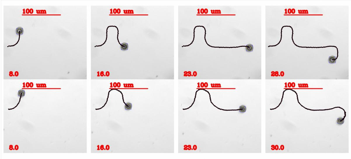
Fig. 9. Snapshots of a different set of *baseline* (top) and *corrected* (bottom) experiments, taken approximately 8 seconds apart and showing the  $\mu$ bot with the position history overlaid.
