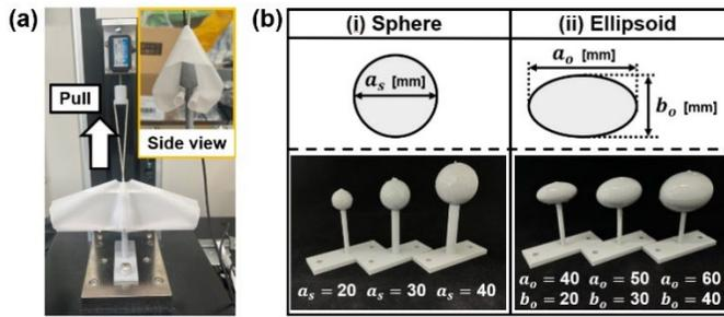
Fig. 9. Experimental setup for evaluation of grasping force. (a) Grasping test. (b) Grasping object.
