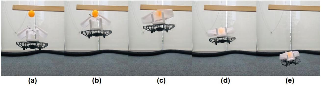
Fig. 14. Grasping experiment equipped with a quadcopter. (a) Ascent process to the object. (b) Contact to the object to grasp. (c) Initiation of grip through contact-trigger activation. (d)-(e) Descent towards the destination.
