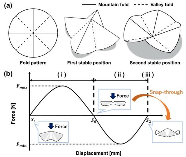
Fig. 4. Mechanism of bistable structure. (a) Water bomb structure. Bistable structures can be imparted to a sheet by alternately folding it in mountain and valley folds in a circular manner. (b) Principle.
