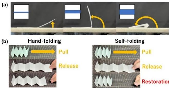
Fig. 2. Characteristic Mechanical property of the self-folded paper. (a) Control of folding angle through variation of printing line width. (b) Elastic memory characteristics to hinge sections of the self-folded paper.
