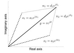
Fig. 1. Consider y which could result from many different speech and noise DFT-coefficient pairs, for example,  $s_1 + n_1$  or  $s_2 + n_2$ . Under Assumptions 1) and 3),  $f_{Y|S}(y|s)$  is given by (2) and depends only on the magnitude d = |y-s| of the noise DFT coefficient n. Therefore,  $f_{Y|S}(y|s_1)$  equals  $f_{Y|S}(y|s_2)$  when  $d_1 = d_2$ .
