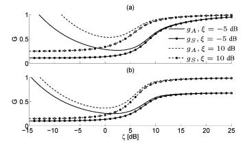
Fig. 2. Complex-DFT and DFT-magnitude gain curves for  $\xi = -5$  dB and  $\xi = 10$  dB, for (a)  $\gamma = 1, \nu = 0.6, K = 20$  and (b)  $\gamma = 2, \nu = 0.15$ .
